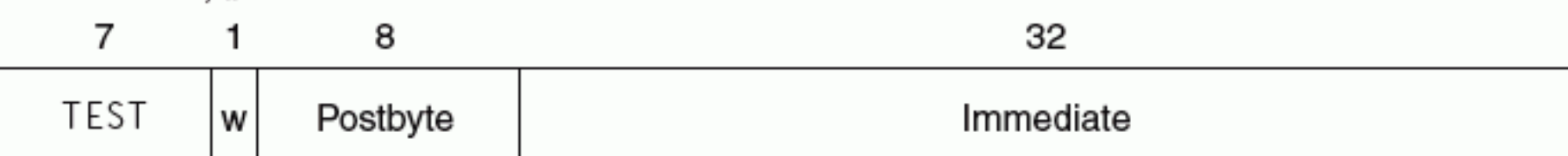
FIGURE 2.45 Typical IA-32 instruction formats. Figure 2.46 shows the encoding of the postbyte. Many instructions contain the 1-bit field w, which says whether the operation is a byte or double word. The d field in MOV is used in instructions that may move to or from memory and shows the direction of the move. The ADD instruction requires 32 bits for the immediate field because in 32-bit mode the immediates are either 8 bits or 32 bits. The immediate field in the TEST is 32 bits long because there is no 8-bit immediate for test in 32-bit mode. Overall, instructions may vary from 1 to 17 bytes in length. The long length comes from extra 1-byte prefixes, having both a 4-byte immediate and a 4-byte displacement address, using an opcode of 2 bytes, and using the scaled index mode specifier, which adds another byte.
