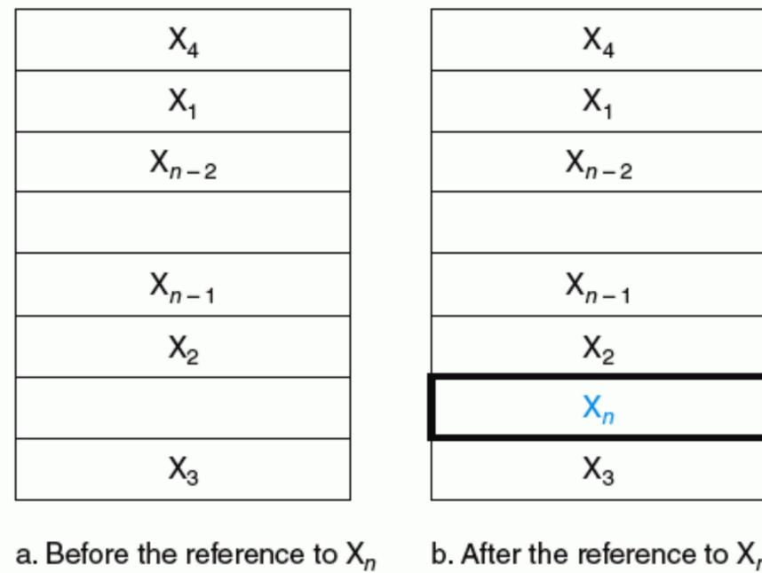
**FIGURE 7.4** The cache just before and just after a reference to a word  $X_n$  that is not initially in the cache. This reference causes a miss that forces the cache to fetch  $X_n$  from memory and insert it into the cache.
