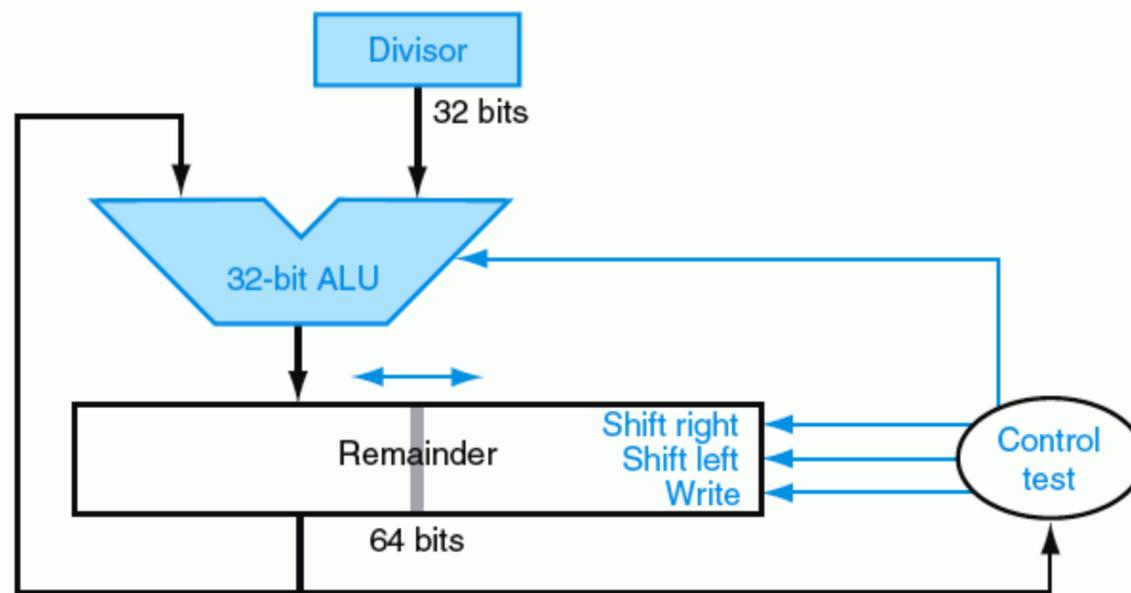
**FIGURE 3.13 An improved version of the division hardware.** The Divisor register, ALU, and Quotient register are all 32 bits wide, with only the Remainder register left at 64 bits. Compared to Figure 3.10, the ALU and Divisor registers are halved and the remainder is shifted left. This version also combines the Quotient register with the right half of the Remainder register.
