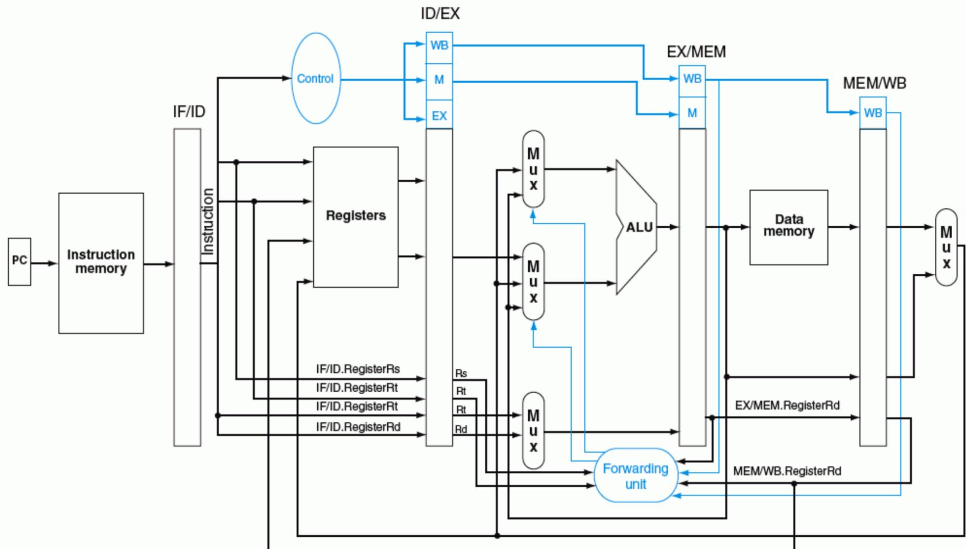
**FIGURE 6.32** The datapath modified to resolve hazards via forwarding. Compared with the datapath in Figure 6.27 on page 404, the additions are the multiplexers to the inputs to the ALU. This figure is a more stylized drawing, however, leaving out details from the full datapath such as the branch hardware and the sign extension hardware.
