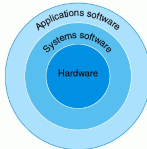
**FIGURE 1.3** A simplified view of hardware and software as hierarchical layers, shown as concentric circles with hardware in the center and applications software outermost. In complex applications there are often multiple layers of application software as well. For example, a database system may run on top of the systems software hosting an application, which in turn runs on top of the database.
