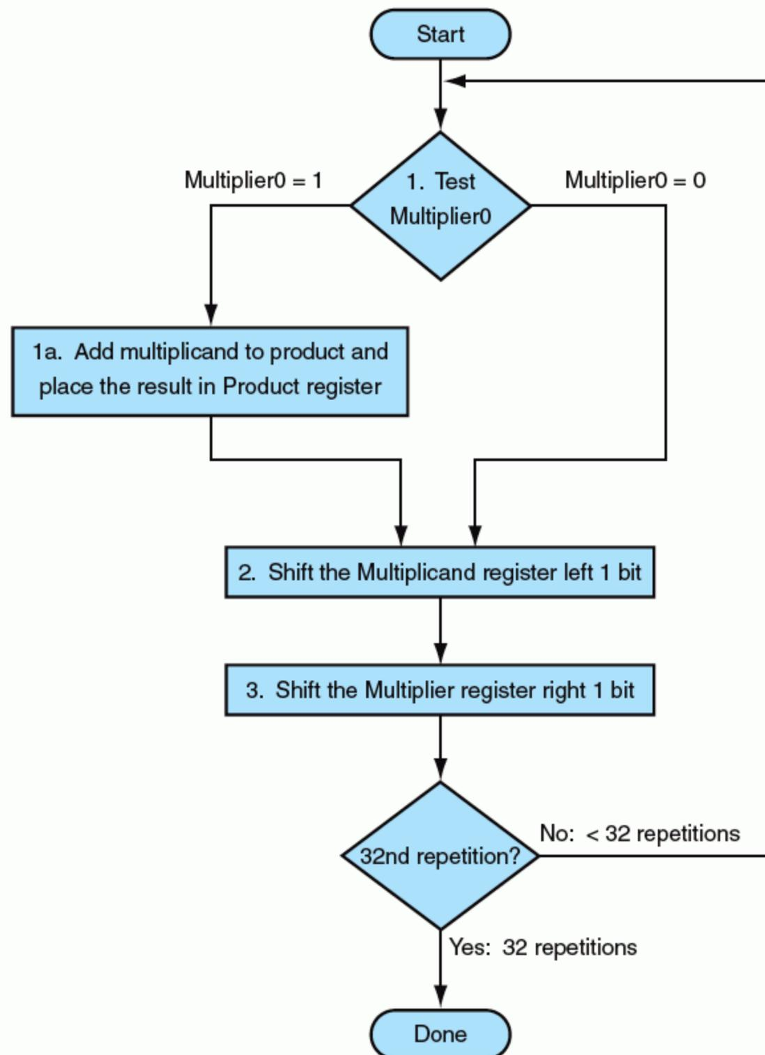
**FIGURE 3.6** The first multiplication algorithm, using the hardware shown in Figure 3.5. If the least significant bit of the multiplier is 1, add the multiplicand to the product. If not, go to the next step. Shift the multiplicand left and the multiplier right in the next two steps. These three steps are repeated 32 times.
