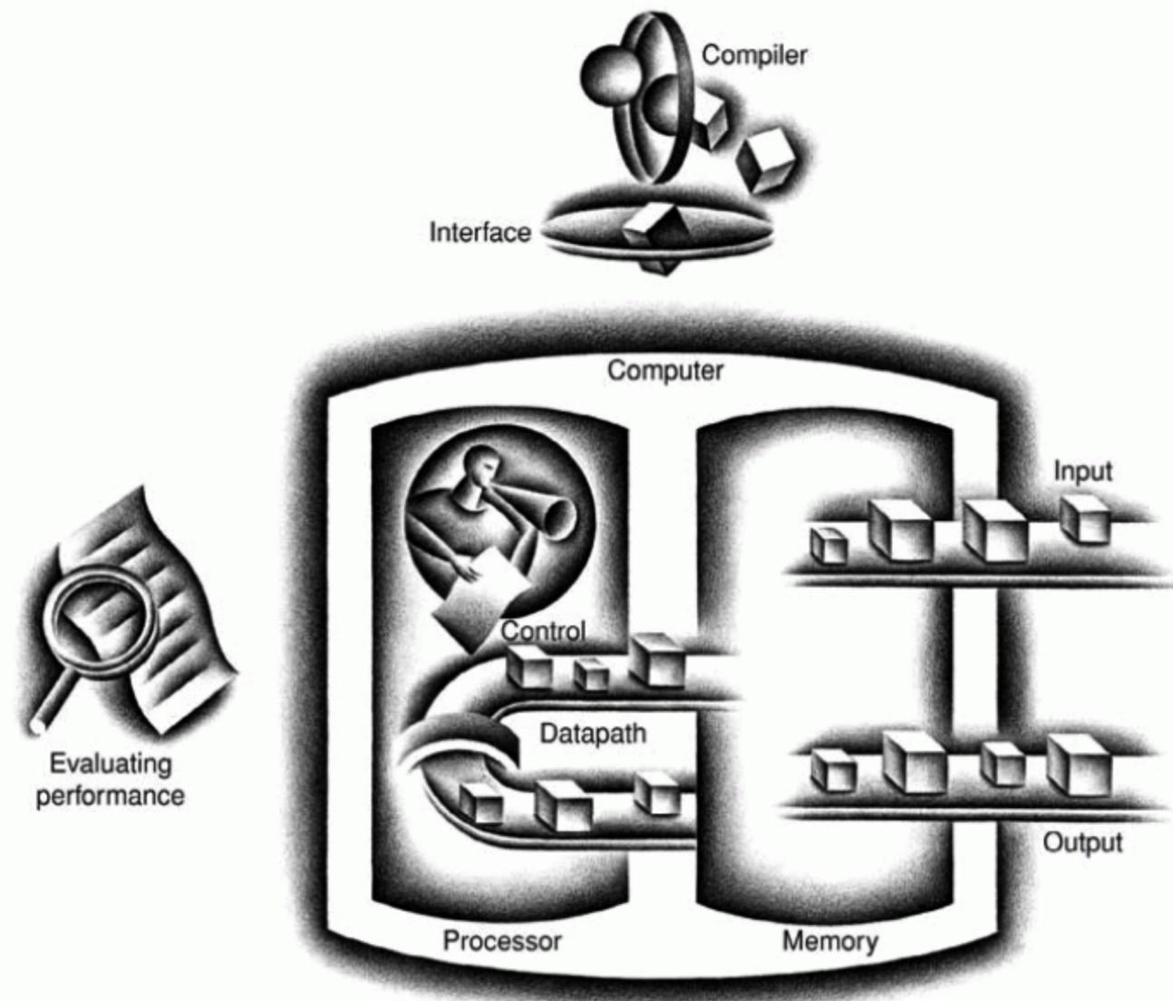
**FIGURE 1.5 The organization of a computer, showing the five classic components.** The processor gets instructions and data from memory. Input writes data to memory, and output reads data from memory. Control sends the signals that determine the operations of the datapath, memory, input, and output.
