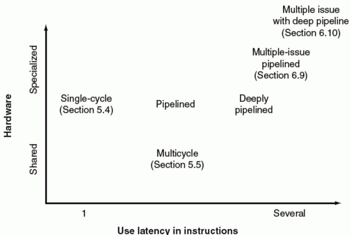
**FIGURE 6.53** The basic relationship between the datapaths in Figure 6.52. Notice that the  $x$ -axis is use latency in instructions, which is what determines the ease of keeping the pipeline full. The pipelined datapath is shown as multiple clock cycles for instruction latency because the execution time of an instruction is not shorter; it's the instruction throughput that is improved.
