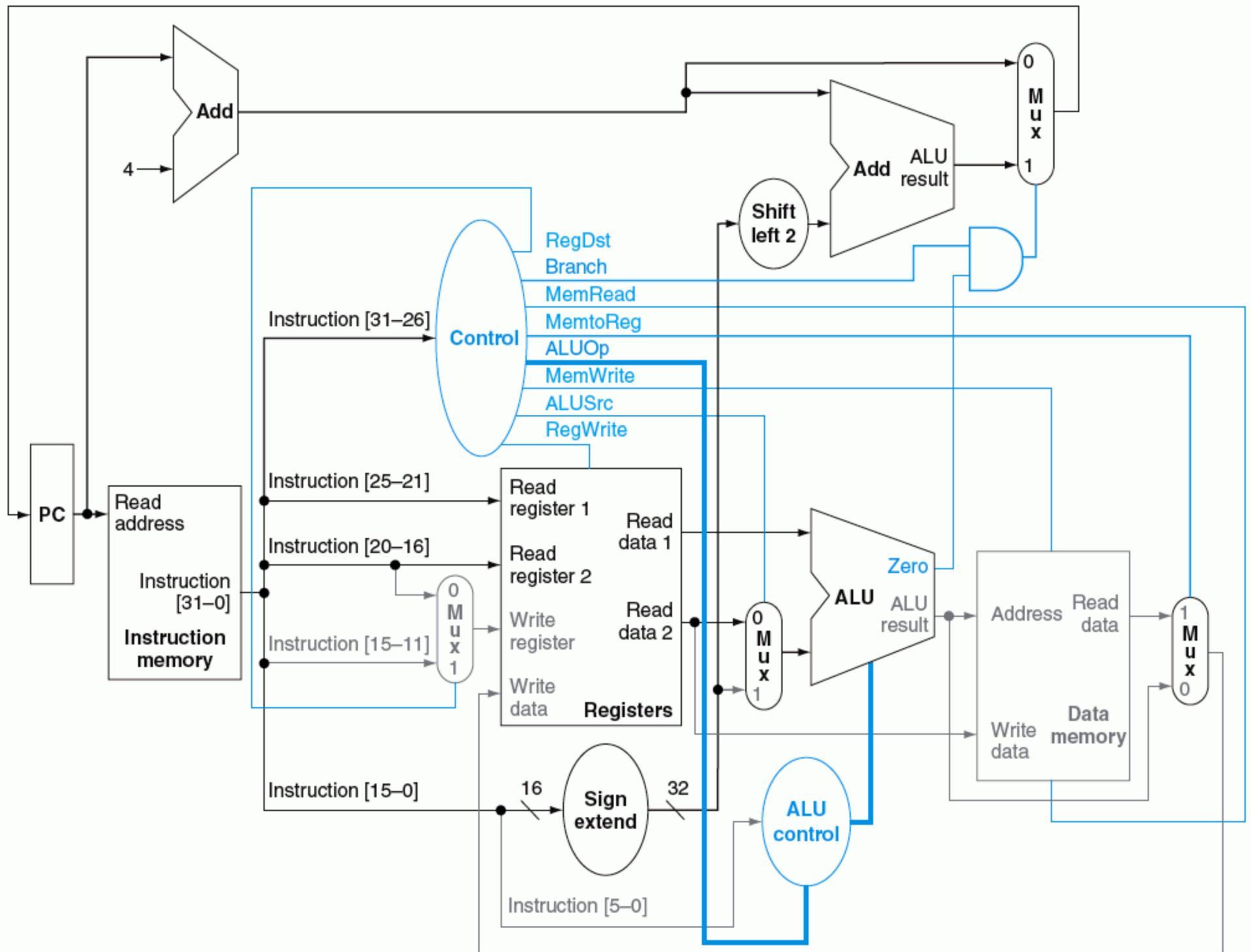
**FIGURE 5.21** The datapath in operation for a branch equal instruction. The control lines, datapath units, and connections that are active are highlighted. After using the register file and ALU to perform the compare, the Zero output is used to select the next program counter from between the two candidates.
