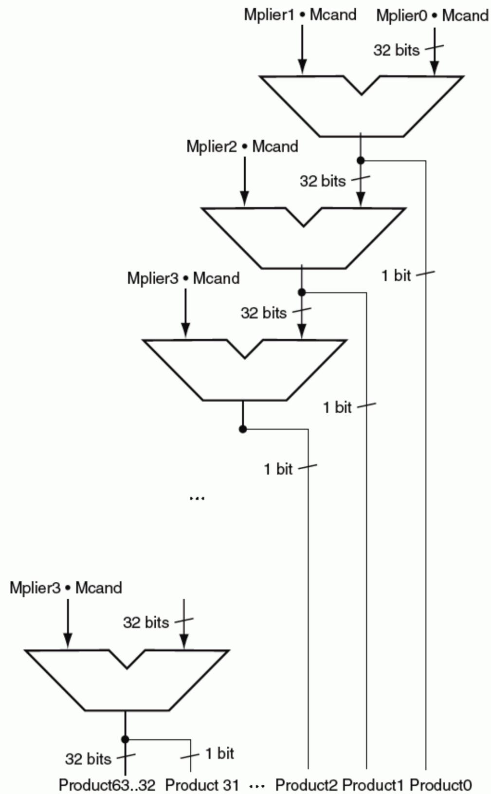
**FIGURE 3.9 Fast multiplication hardware.** Rather than use a single 32-bit adder 32 times, this hardware “unrolls the loop” to use 32 adders. Each adder produces a 32-bit sum and a carry out. The least significant bit is a bit of the product, and the carry out and the upper 31 bits of the sum are passed along to the next adder.
