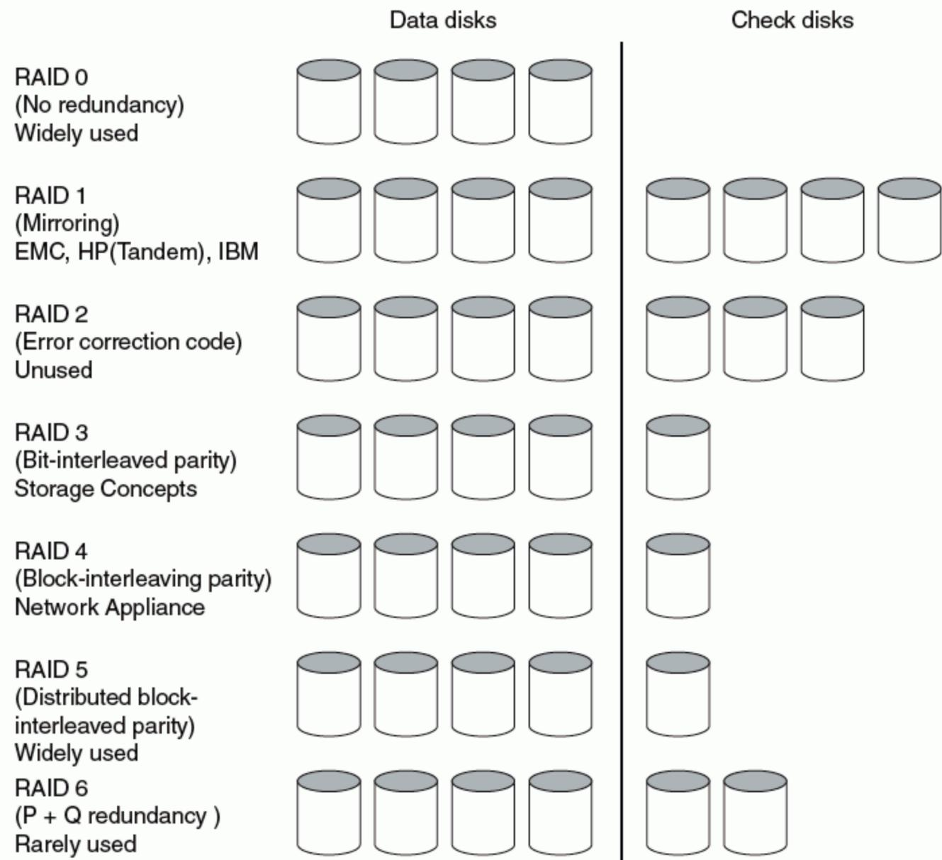
**FIGURE 8.6 RAID for an example of four data disks showing extra check disks per RAID level and companies that use each level.** Figures 8.7 and 8.8 explain the difference between RAID 3, RAID 4, and RAID 5.
