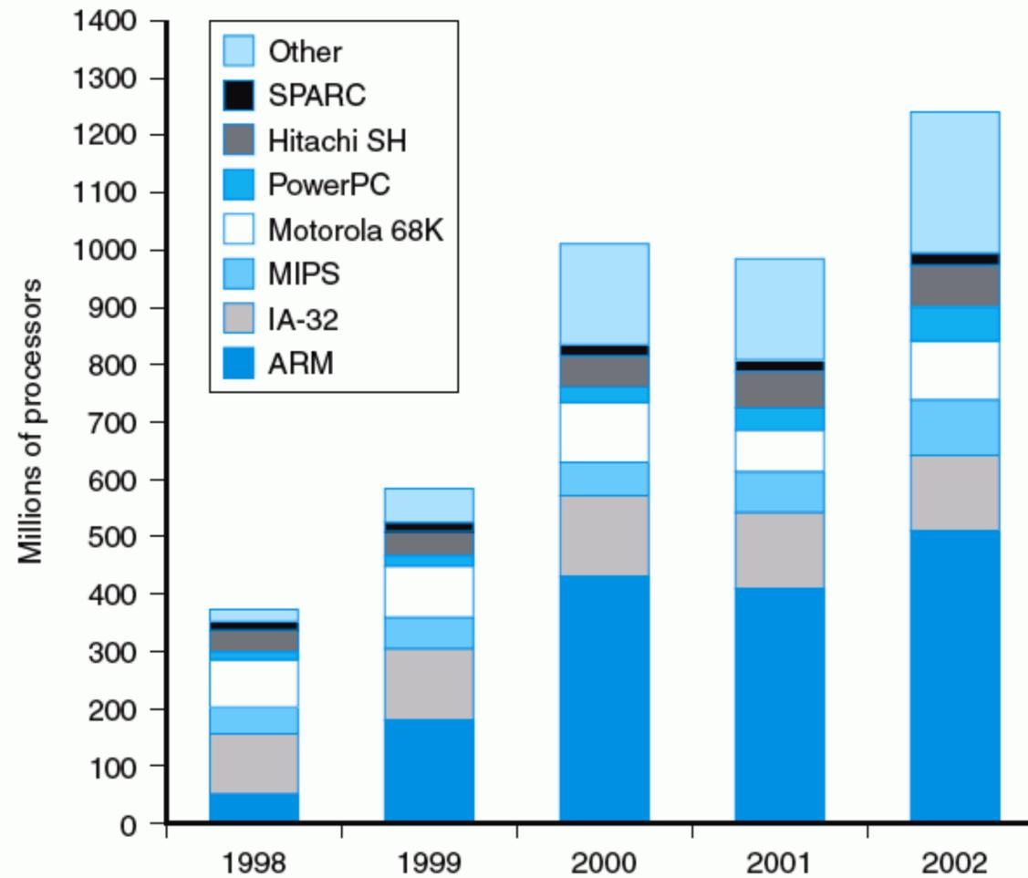
**FIGURE 1.2 Sales of microprocessors between 1998 and 2002 by instruction set architecture combining all uses.** The “other” category refers to processors that are either application-specific or customized architectures. In the case of ARM, roughly 80% of the sales are for cell phones, where an ARM core is used in conjunction with application-specific logic on a chip.
