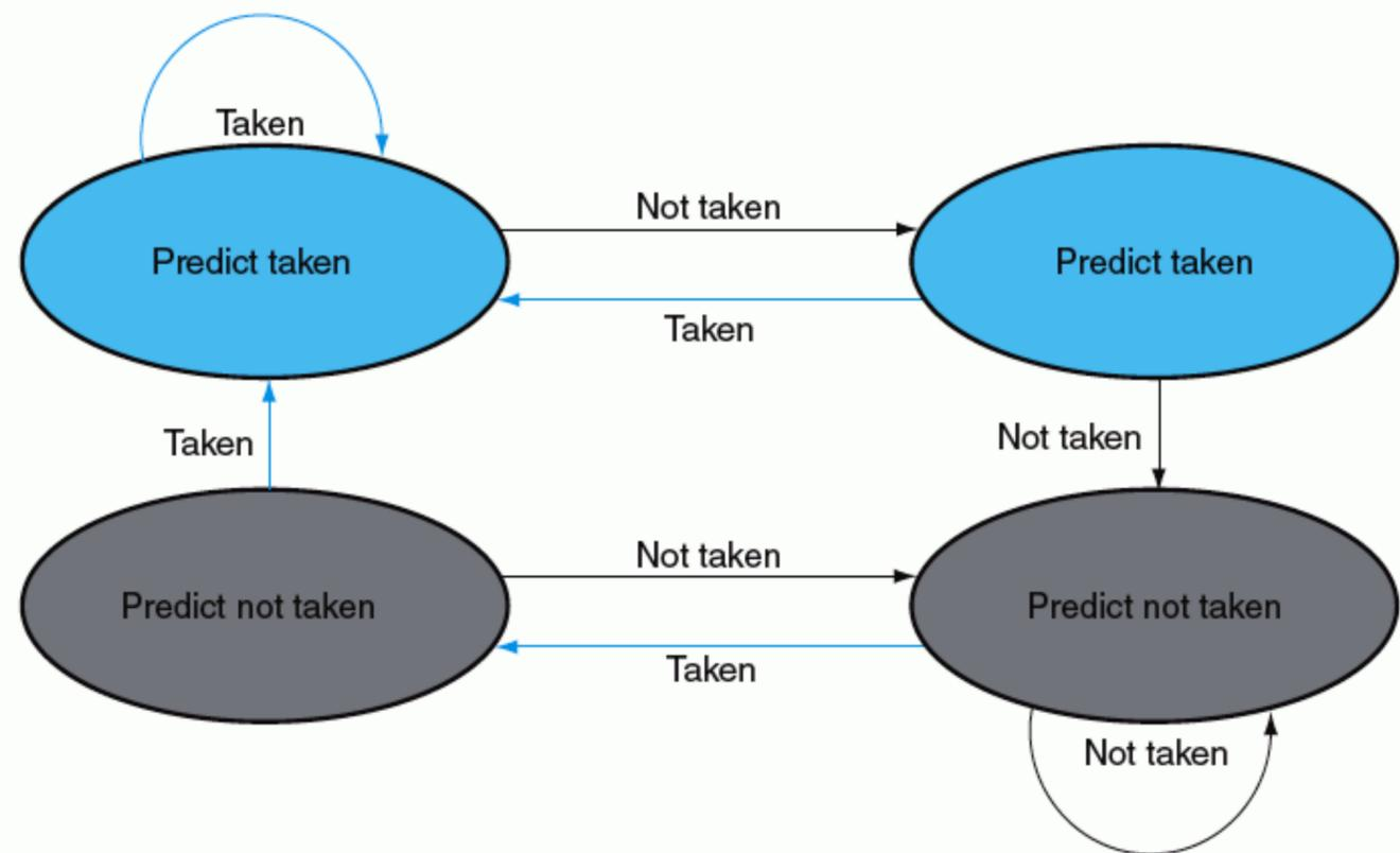
**FIGURE 6.39** The states in a 2-bit prediction scheme. By using 2 bits rather than 1, a branch that strongly favors taken or not taken—as many branches do—will be mispredicted only once. The 2 bits are used to encode the four states in the system. The two-bit scheme is a general instance of a counter-based predictor, which is incremented when the prediction is accurate and decremented otherwise, and uses the midpoint of its range as the division between taken and not taken.
