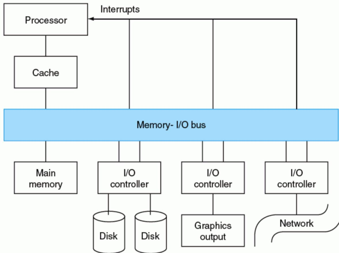
**FIGURE 8.1 A typical collection of I/O devices.** The connections between the I/O devices, processor, and memory are usually called *buses*. Communication among the devices and the processor use both interrupts and protocols on the bus, as we will see in this chapter. Figure 8.11 on page 585 shows the organization for a desktop PC.
