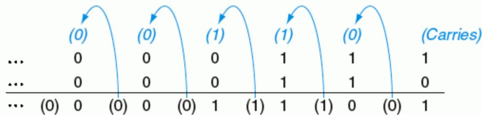
**FIGURE 3.2 Binary addition, showing carries from right to left.** The rightmost bit adds 1 to 0, resulting in the sum of this bit being 1 and the carry out from this bit being 0. Hence, the operation for the second digit to the right is  $0 + 1 + 1$ . This generates a 0 for this sum bit and a carry out of 1. The third digit is the sum of  $1 + 1 + 1$ , resulting in a carry out of 1 and a sum bit of 1. The fourth bit is  $1 + 0 + 0$ , yielding a 1 sum and no carry.
