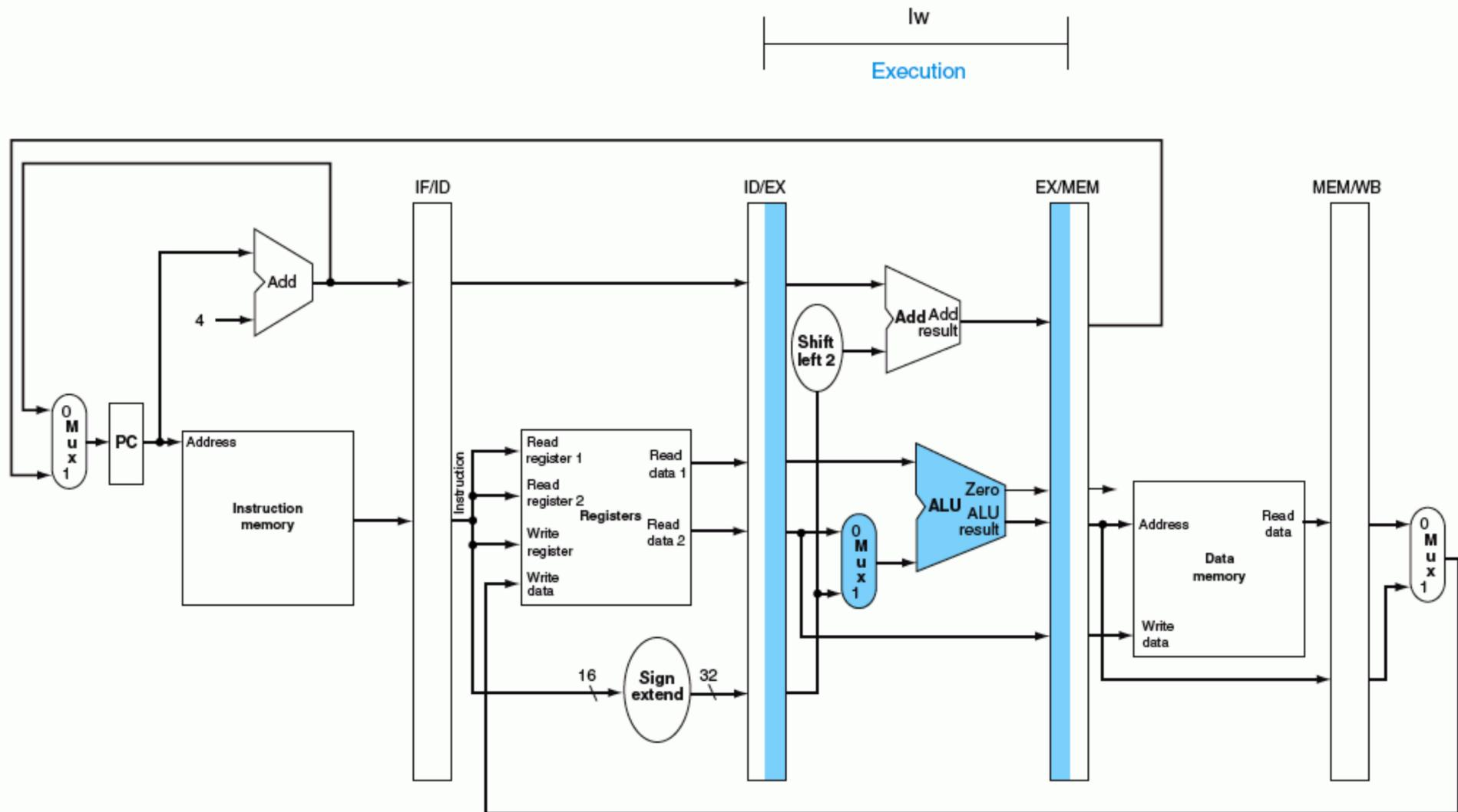
**FIGURE 6.13** EX: the third pipe stage of a load instruction, highlighting the portions of the datapath in Figure 6.11 used in this pipe stage. The register is added to the sign-extended immediate, and the sum is placed in the EX/MEM pipeline register.
