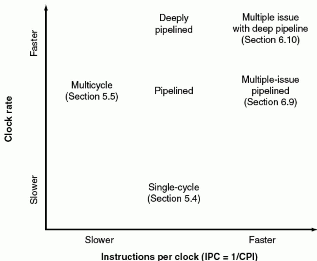
**FIGURE 6.52** The performance consequences of simple (single-cycle) datapath and multicycle datapath from Chapter 5 and the pipelined execution model in Chapter 6. Remember that CPU performance is a function of IPC times clock rate, and hence moving to the upper right increases performance. Although the instructions per clock cycle is slightly larger in the simple datapath, the pipelined datapath is close, and it uses a clock rate as fast as the multicycle datapath.
