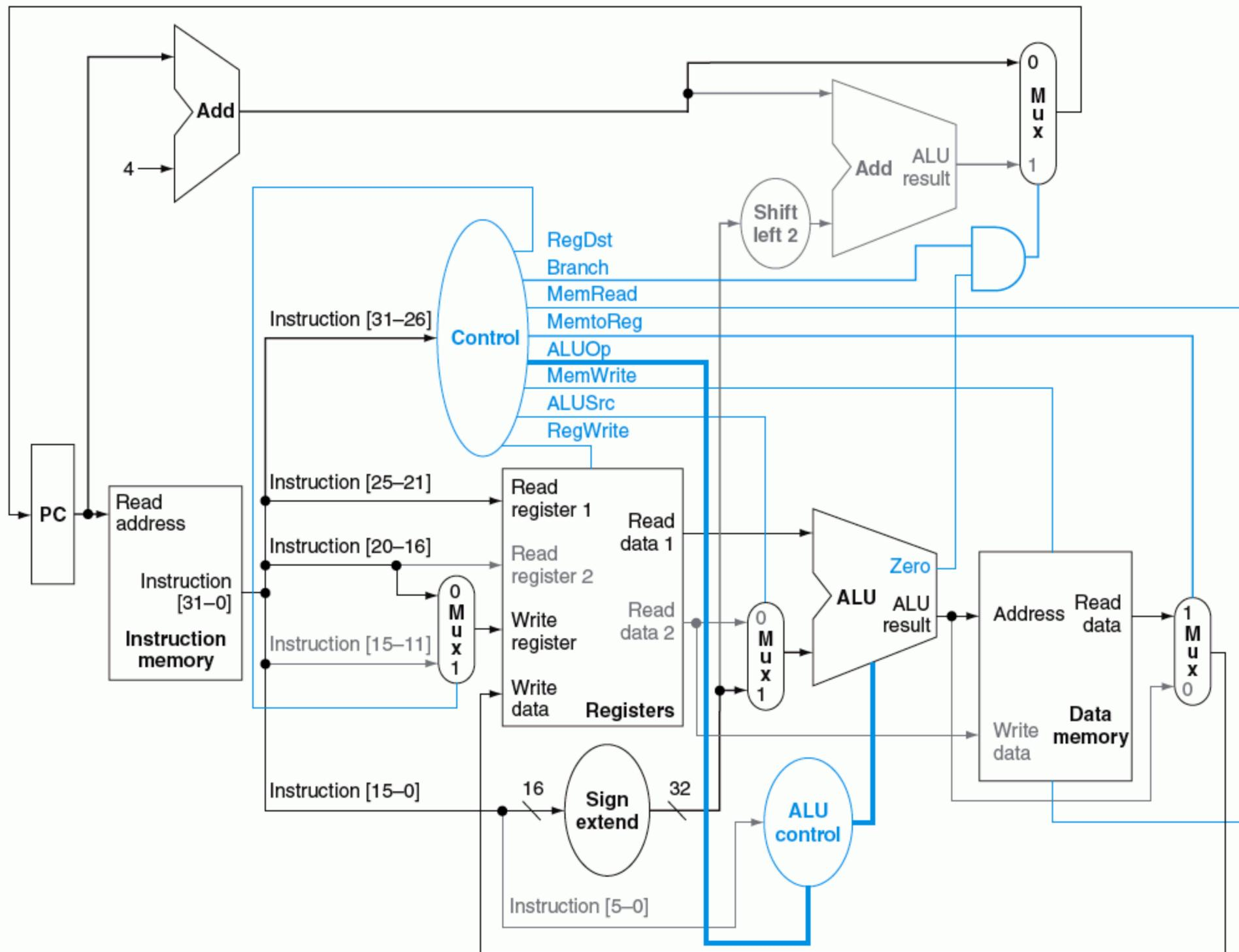
**FIGURE 5.20** The datapath in operation for a load instruction. The control lines, datapath units, and connections that are active are highlighted. A store instruction would operate very similarly. The main difference would be that the memory control would indicate a write rather than a read, the second register value read would be used for the data to store, and the operation of writing the data memory value to the register file would not occur.
