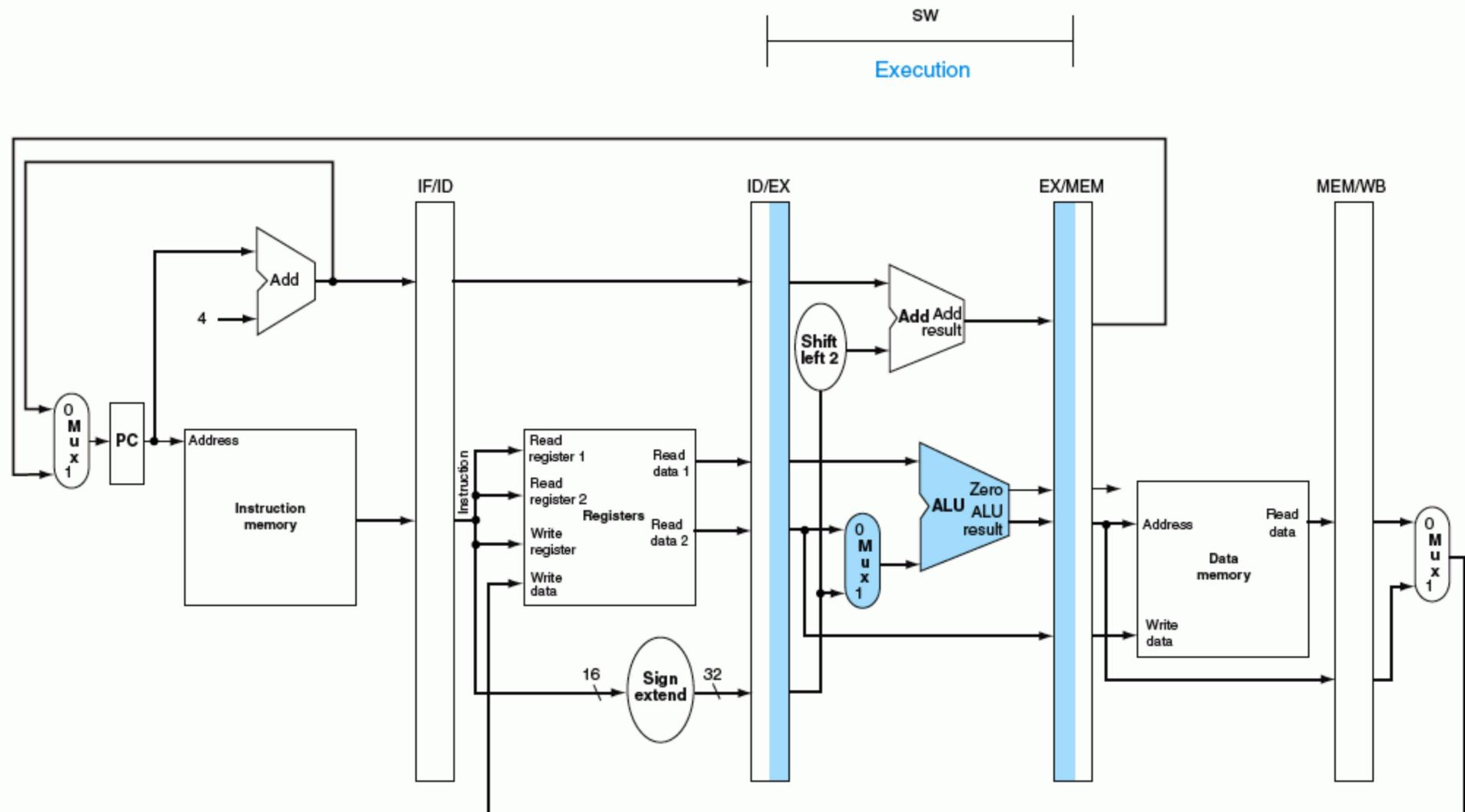
**FIGURE 6.15 EX: the third pipe stage of a store instruction.** Unlike the third stage of the load instruction in Figure 6.13, the second register value is loaded into the EX/MEM pipeline register to be used in the next stage. Although it wouldn't hurt to always write this second register into the EX/MEM pipeline register, we write the second register only on a store instruction to make the pipeline easier to understand.
