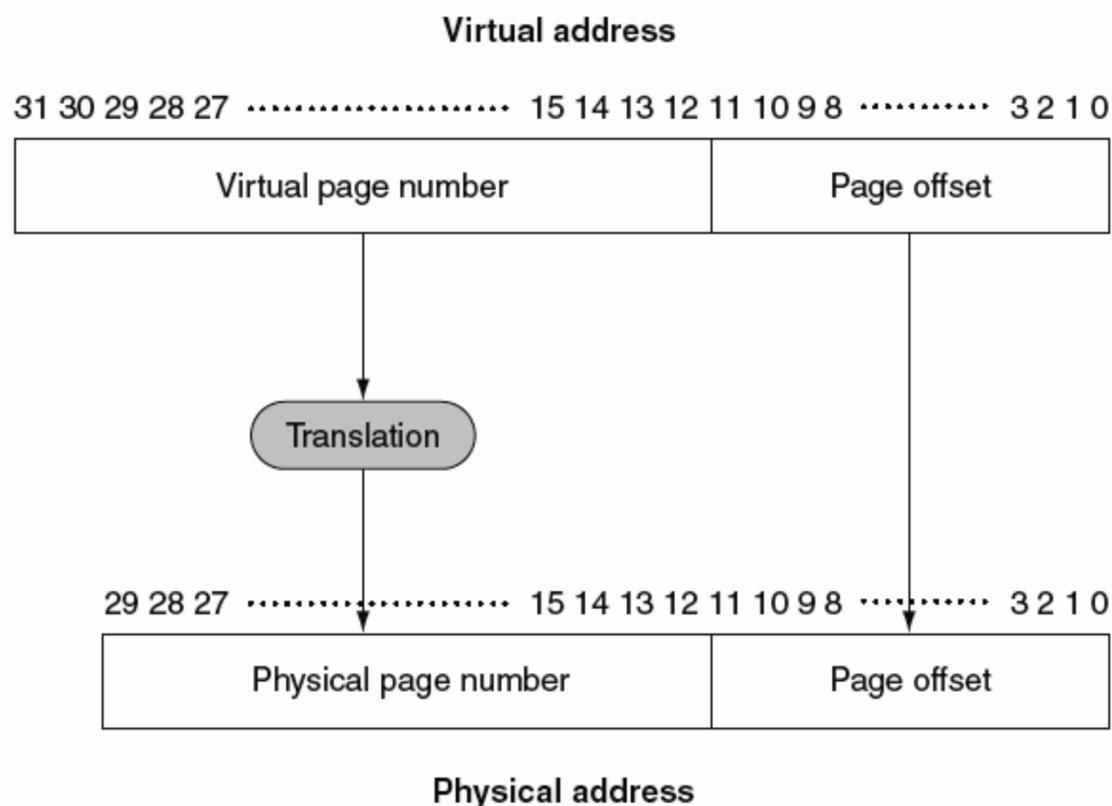
**FIGURE 7.20 Mapping from a virtual to a physical address.** The page size is  $2^{12} = 4$  KB. The number of physical pages allowed in memory is  $2^{18}$ , since the physical page number has 18 bits in it. Thus, main memory can have at most 1 GB, while the virtual address space is 4 GB.
