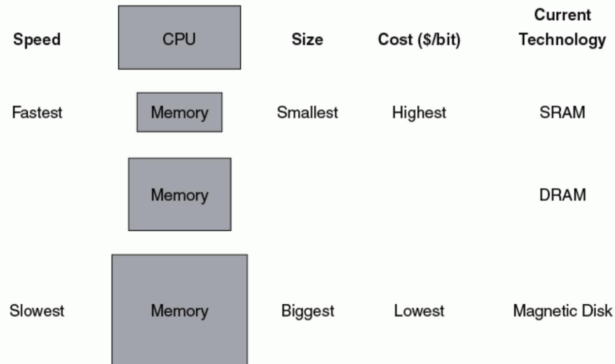
**FIGURE 7.1 The basic structure of a memory hierarchy.** By implementing the memory system as a hierarchy, the user has the illusion of a memory that is as large as the largest level of the hierarchy, but can be accessed as if it were all built from the fastest memory.
