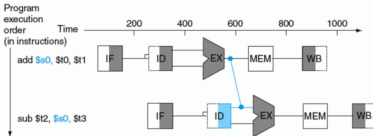
**FIGURE 6.5** Graphical representation of forwarding. The connection shows the forwarding path from the output of the *EX* stage of *add* to the input of the *EX* stage for *sub*, replacing the value from register *\$s0* read in the second stage of *sub*.
