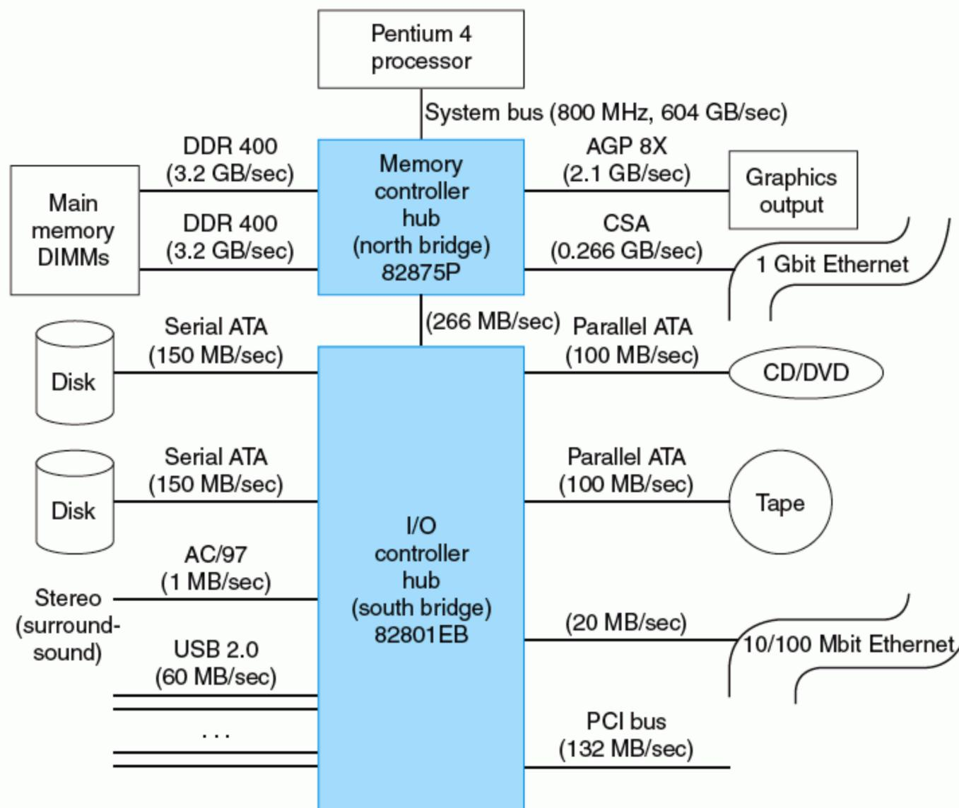
**FIGURE 8.11** Organization of the I/O system on a Pentium 4 PC using the Intel 875 chip set. Note that the maximum transfer rate between the north bridge (memory hub) and south bridge (I/O hub) is 266 MB/sec, which is why Intel put the AGP bus and Gigabit Ethernet on the north bridge.
