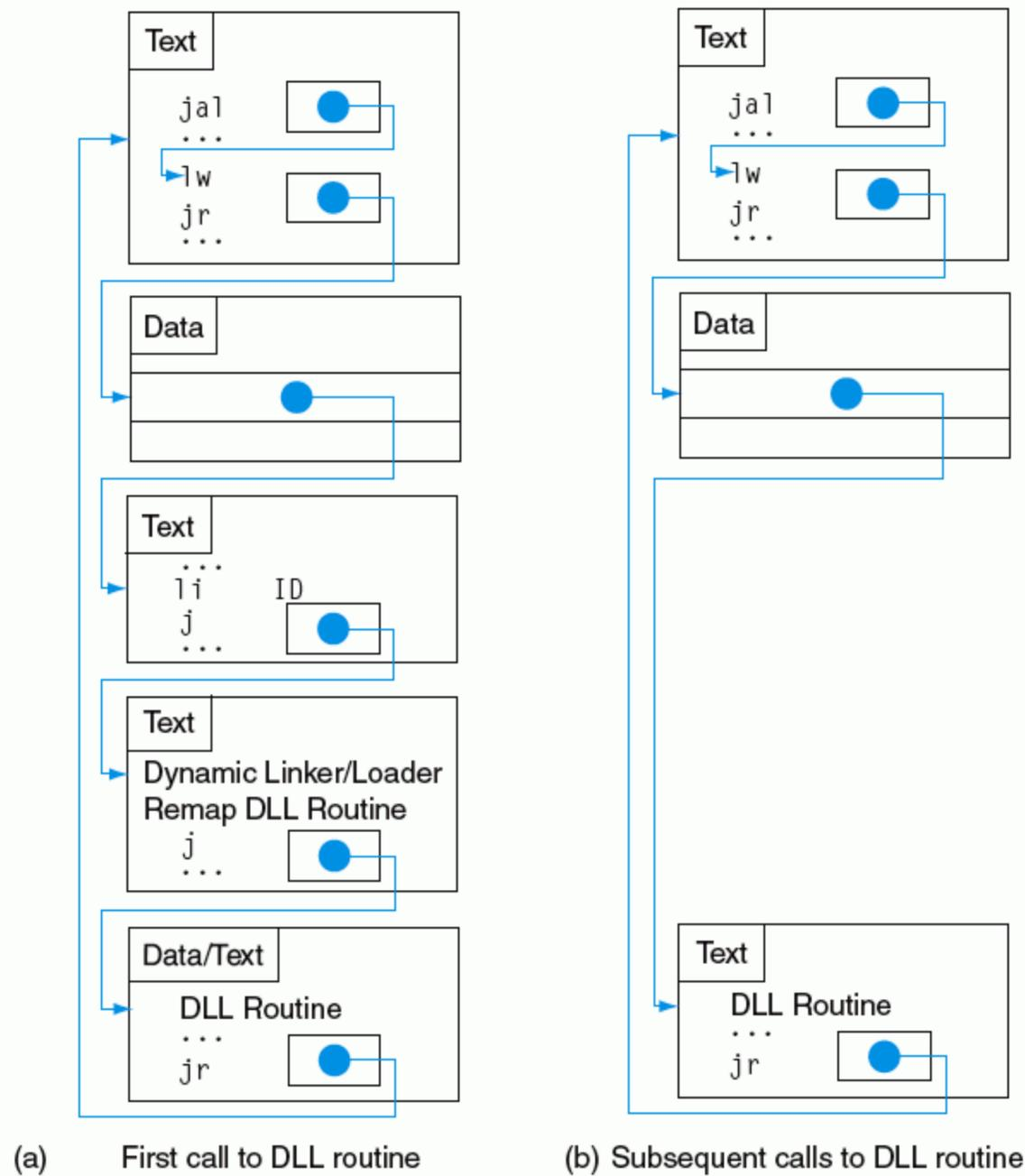
**FIGURE 2.29 Dynamically linked library via lazy procedure linkage.** (a) Steps for the first time a call is made to the DLL routine. (b) The steps to find the routine, remap it, and link it are skipped on subsequent calls. As we will see in Chapter 7, the operating system may avoid copying the desired routine by remapping it using virtual memory management.
