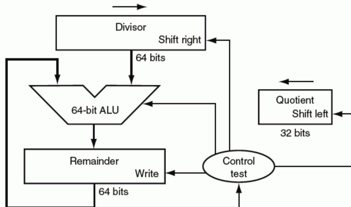
**FIGURE 3.10 First version of the division hardware.** The Divisor register, ALU, and Remainder register are all 64 bits wide, with only the Quotient register being 32 bits. The 32-bit divisor starts in the left half of the Divisor register and is shifted right 1 bit on each iteration. The remainder is initialized with the dividend. Control decides when to shift the Divisor and Quotient registers and when to write the new value into the Remainder register.
