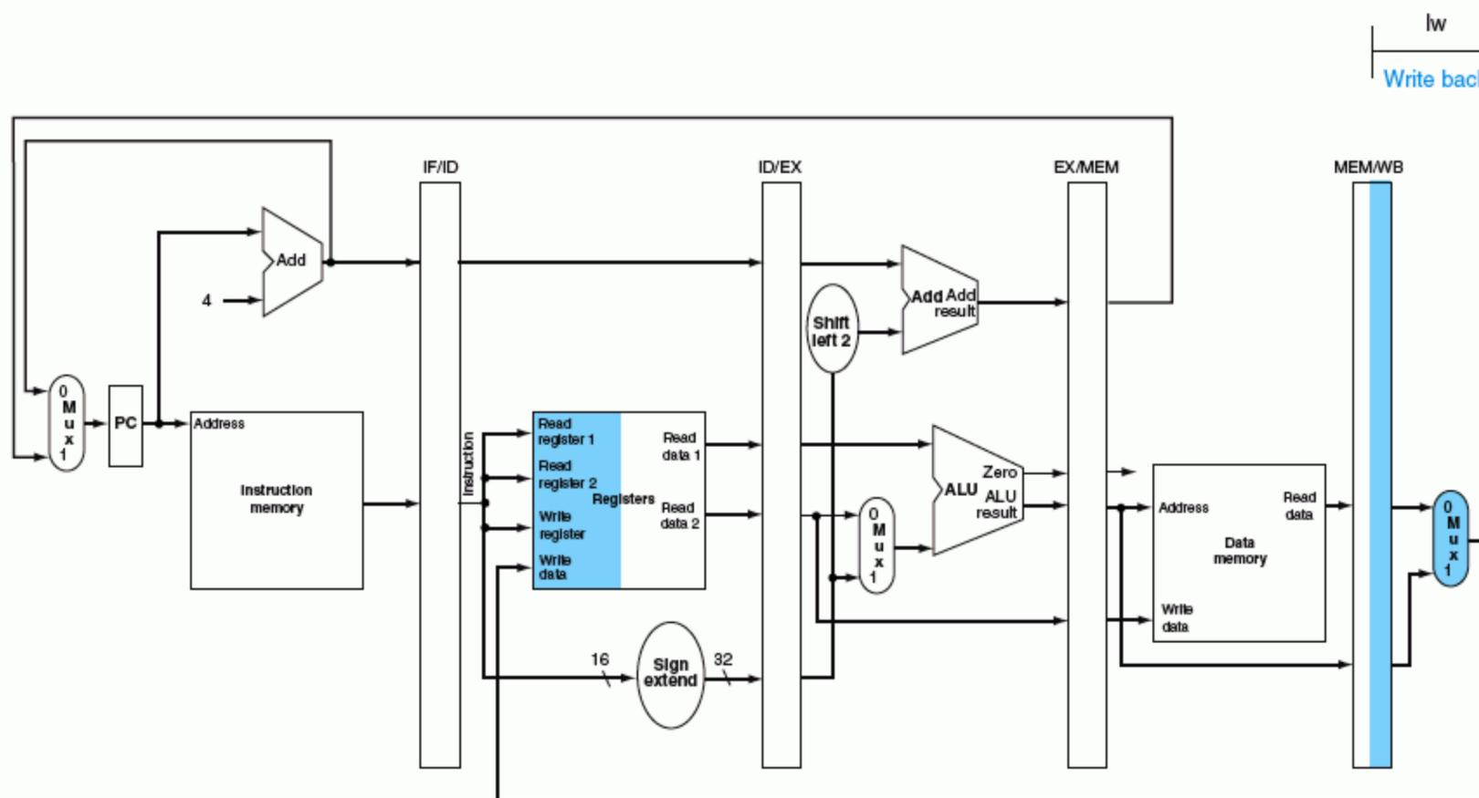
**FIGURE 6.14 MEM and WB: the fourth and fifth pipe stages of a load instruction, highlighting the portions of the datapath in Figure 6.11 used in this pipe stage.** Data memory is read using the address in the EX/MEM pipeline registers, and the data is placed in the MEM/WB pipeline register. Next, data is read from the MEM/WB pipeline register and written into the register file in the middle of the datapath.
