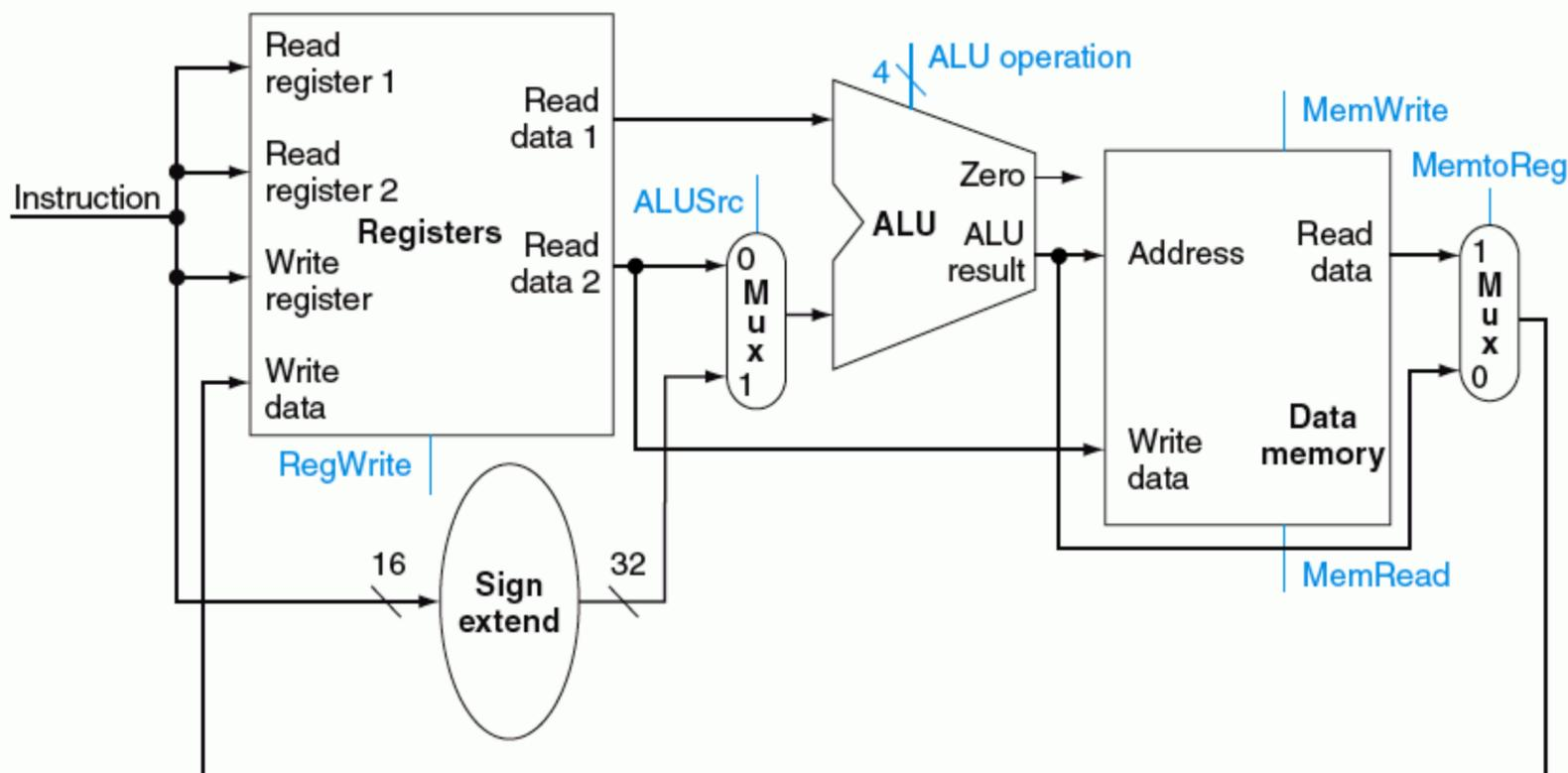
**FIGURE 5.10 The datapath for the memory instructions and the R-type instructions.** This example shows how a single datapath can be assembled from the pieces in Figures 5.7 and 5.8 by adding multiplexors. Two multiplexors are needed, as described as in the example.
