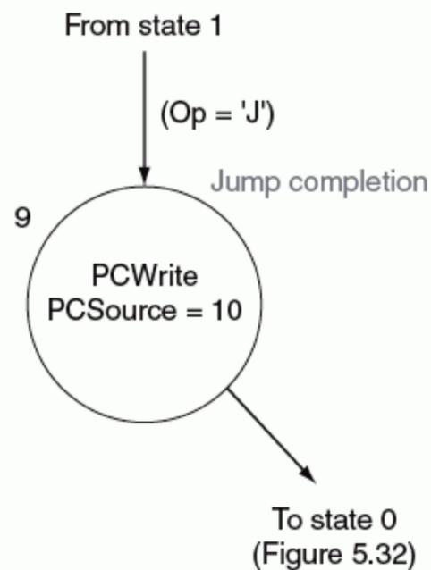
**FIGURE 5.36 The jump instruction requires a single state that asserts two control signals to write the PC with the lower 26 bits of the Instruction register shifted left 2 bits and concatenated to the upper 4 bits of the PC of this instruction.**
