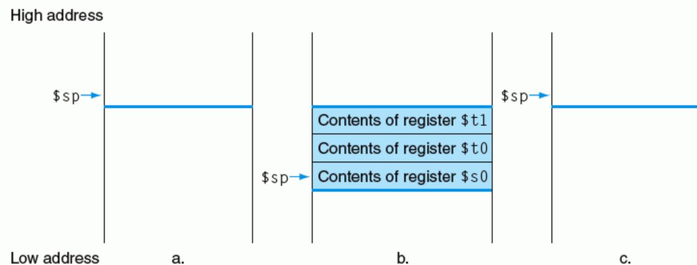
**FIGURE 2.14** The values of the stack pointer and the stack (a) before, (b) during, and (c) after the procedure call. The stack pointer always points to the “top” of the stack, or the last word in the stack in this drawing.
