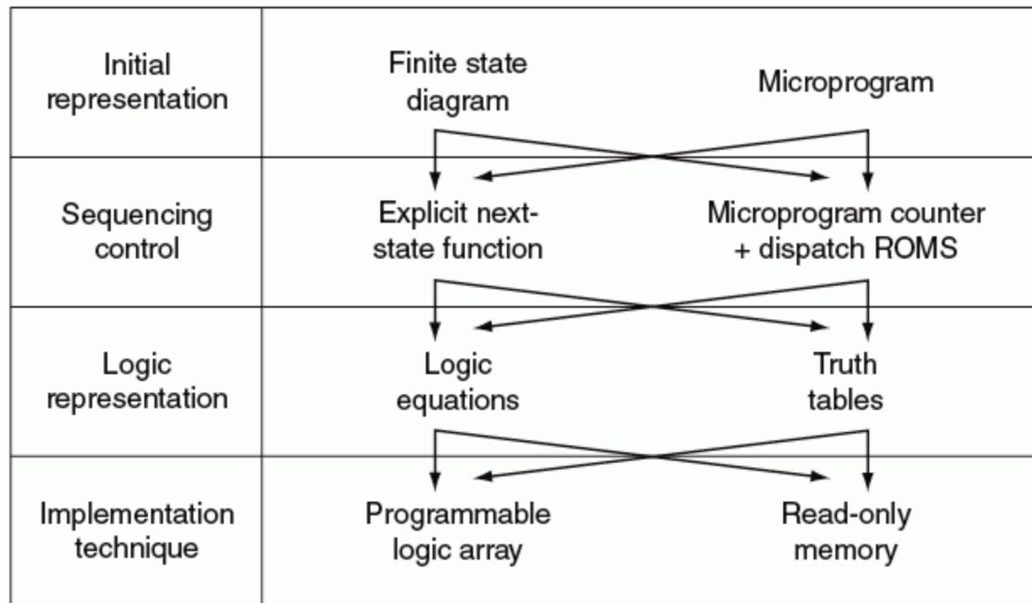
**FIGURE 5.41 Alternative methods for specifying and implementing control.** The arrows indicate possible design paths: any path from the initial representation to the final implementation technology is viable. Traditionally, “hardwired control” means that the techniques on the left-hand side are used, and “microprogrammed control” means that the techniques on the right-hand side are used.
