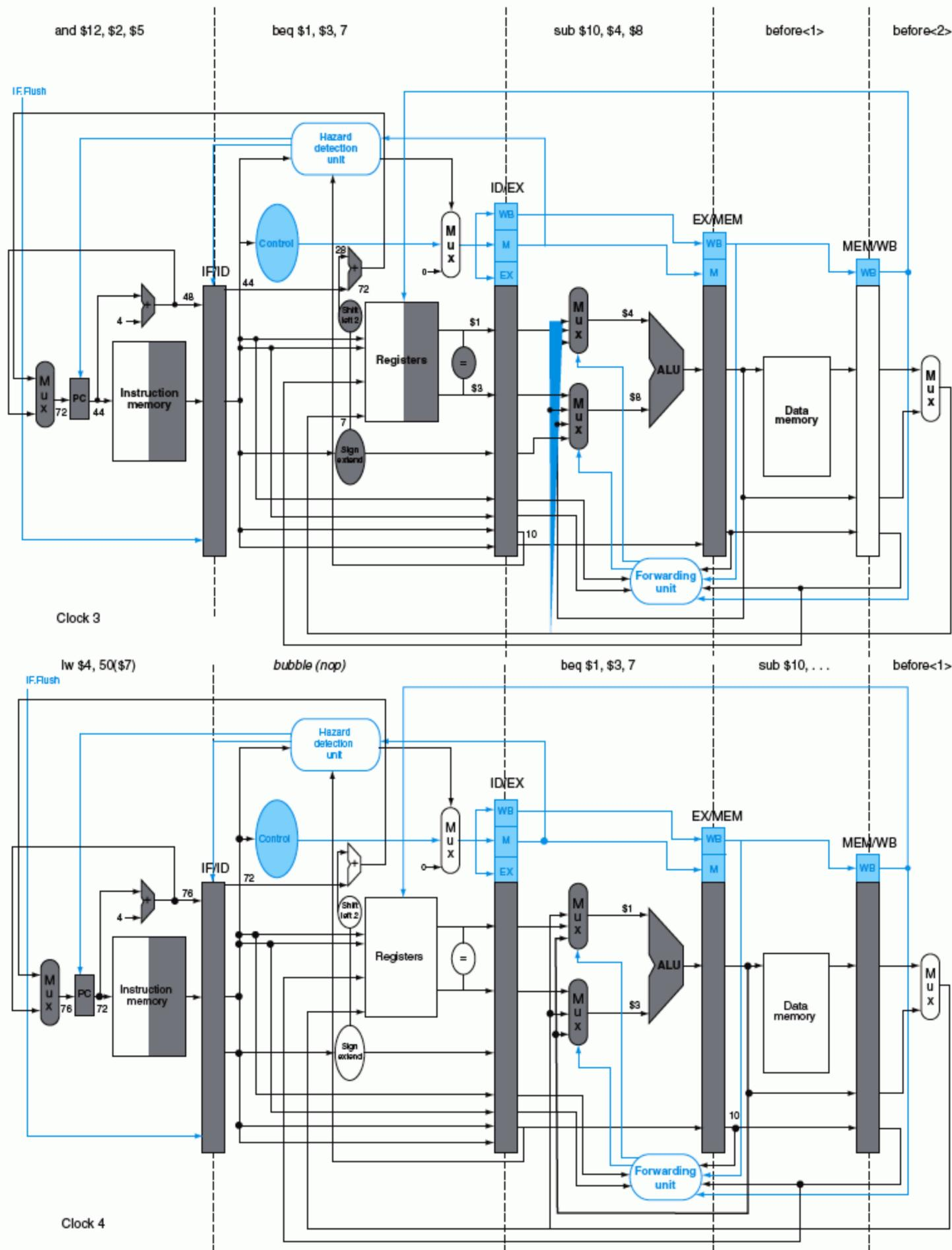
**FIGURE 6.38** The ID stage of clock cycle 3 determines that a branch must be taken, so it selects 72 as the next PC address and zeros the instruction fetched for the next clock cycle. Clock cycle 4 shows the instruction at location 72 being fetched and the single bubble or nop instruction in the pipeline as a result of the taken branch. (Since the nop is really `sll $0, $0, 0`, it's arguable whether or not the ID stage in clock 4 should be highlighted.)
