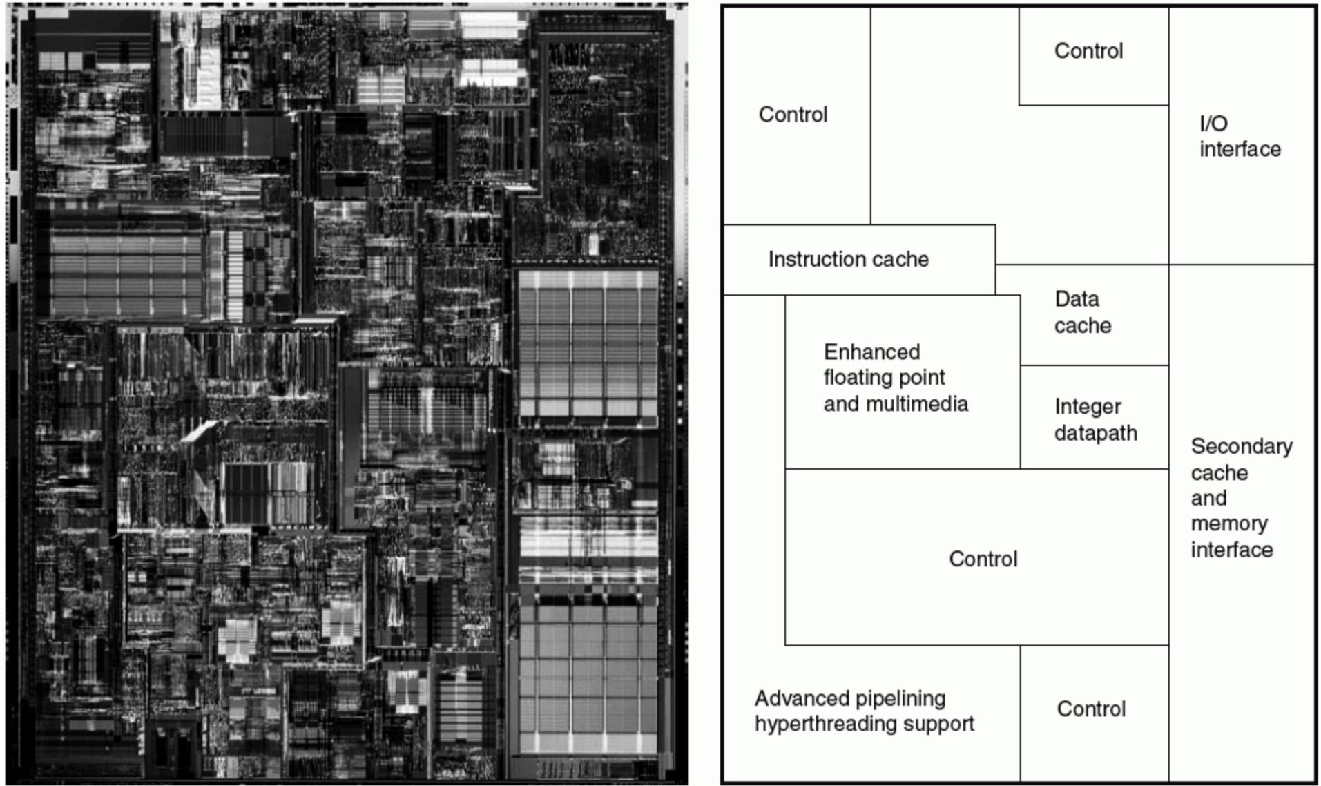
**FIGURE 1.9** Inside the processor chip used on the board shown in Figure 1.8. The left-hand side is a microphotograph of the Pentium 4 processor chip, and the right-hand side shows the major blocks in the processor.
