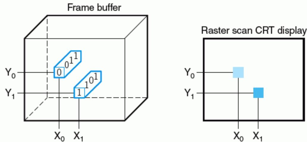
**FIGURE 1.7** Each coordinate in the frame buffer on the left determines the shade of the corresponding coordinate for the raster scan CRT display on the right. Pixel  $(X_0, Y_0)$  contains the bit pattern 0011, which is a lighter shade of gray on the screen than the bit pattern 1101 in pixel  $(X_1, Y_1)$ .
