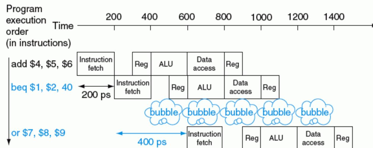
**FIGURE 6.7** Pipeline showing stalling on every conditional branch as solution to control hazards. There is a one-stage pipeline stall, or bubble, after the branch. In reality, the process of creating a stall is slightly more complicated, as we will see in Section 6.6. The effect on performance, however, is the same as would occur if a bubble were inserted.
