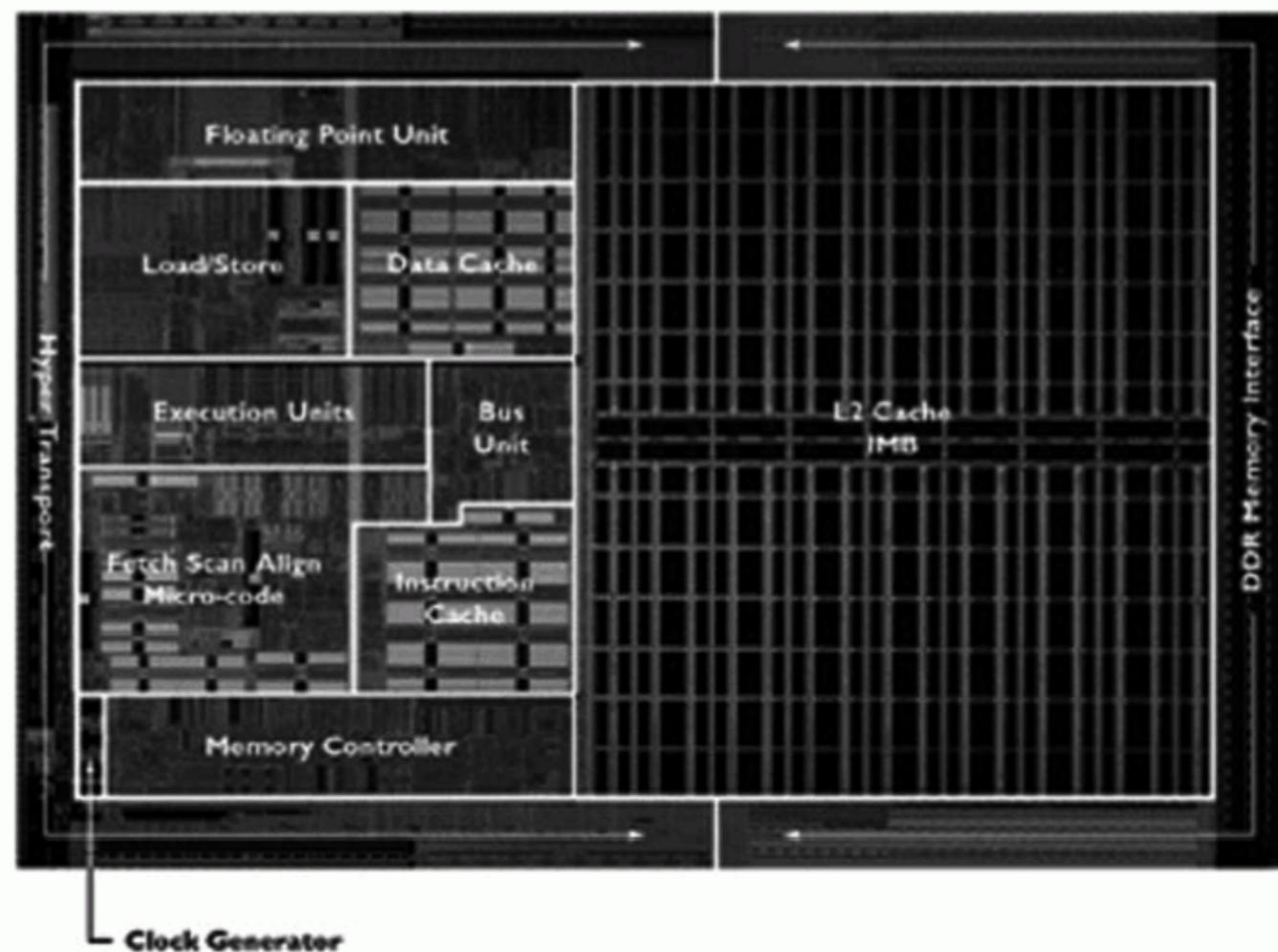
**FIGURE 7.33** An AMD Opteron die processor photo with the components labeled. The L2 cache occupies 42% of the die. The remaining components in order of size are HyperTransport™: 13%, DDR memory: 10%, Fetch/Scan/Align/Microcode: 6%, Memory controller: 4%, FPU: 4%, Instruction cache: 4%, Data cache: 4%, Execution units: 3%, Bus unit: 2%, and clock generator: 0.2%. In a 0.13 technology, this die is 193 mm<sup>2</sup>.
