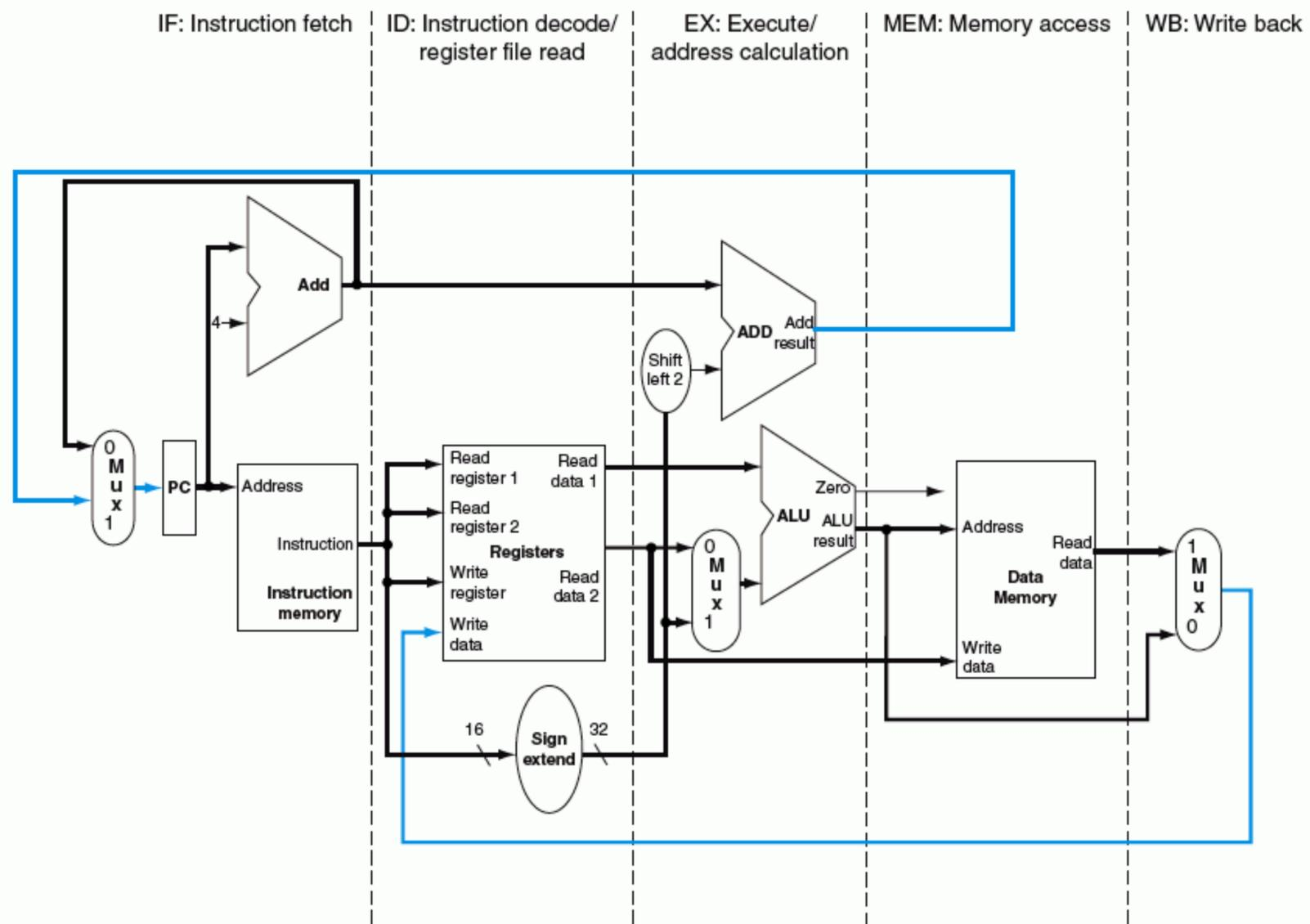
**FIGURE 6.9** The single-cycle datapath from Chapter 5 (similar to Figure 5.17 on page 307). Each step of the instruction can be mapped onto the datapath from left to right. The only exceptions are the update of the PC and the write-back step, shown in color, which sends either the ALU result or the data from memory to the left to be written into the register file. (Normally we use color lines for control, but these are data lines.)
