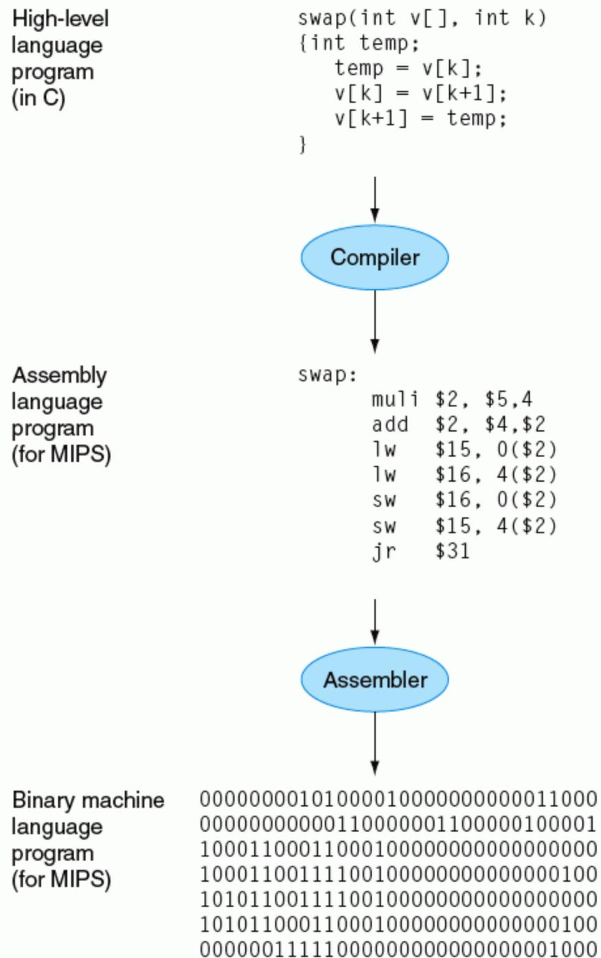
**FIGURE 1.4 C program compiled into assembly language and then assembled into binary machine language.** Although the translation from high-level language to binary machine language is shown in two steps, some compilers cut out the middleman and produce binary machine language directly. These languages and this program are examined in more detail in Chapter 2.
