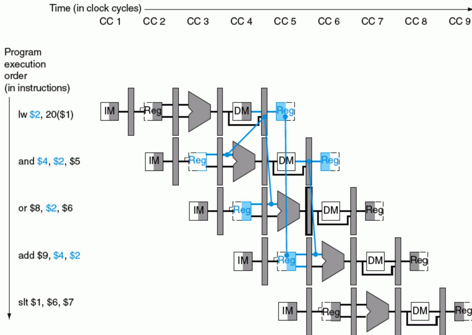
**FIGURE 6.34** A pipelined sequence of instructions. Since the dependence between the load and the following instruction (`and`) goes backwards in time, this hazard cannot be solved by forwarding. Hence, this combination must result in a stall by the hazard detection unit.
