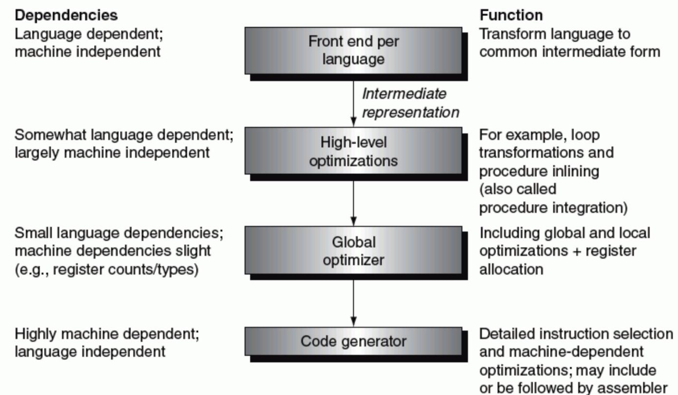
**FIGURE 2.31** The structure of a modern optimizing compiler consists of a numbers of passes or phases. Logically each pass can be thought of as running to completion before the next occurs. In practice, some passes may handle a procedure at a time, essentially interleaving with another pass.
