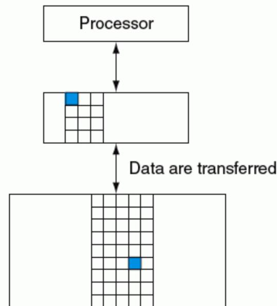
**FIGURE 7.2** Every pair of levels in the memory hierarchy can be thought of as having an upper and lower level. Within each level, the unit of information that is present or not is called a *block*. Usually we transfer an entire block when we copy something between levels.
