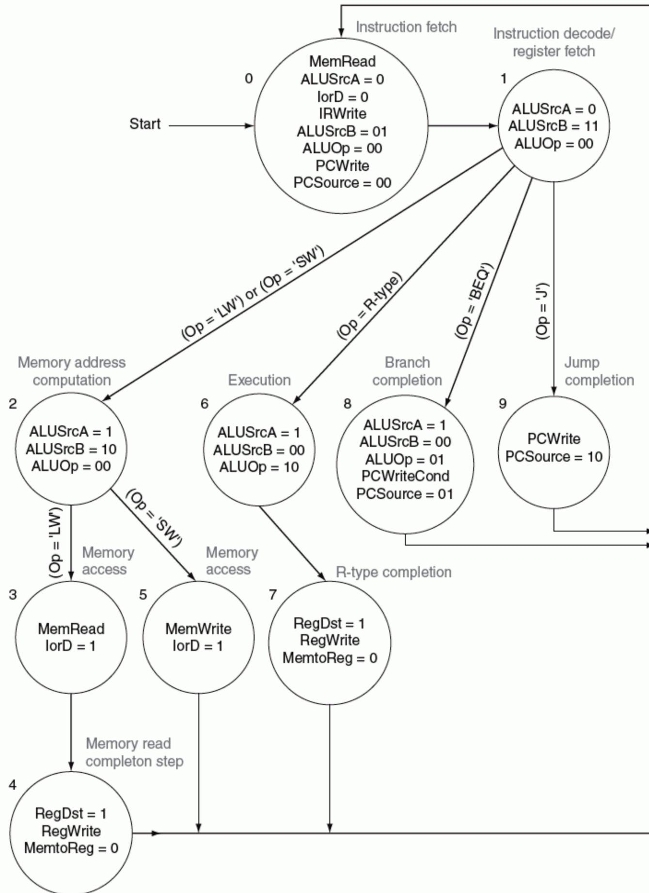
**FIGURE 5.38** The complete finite state machine control for the datapath shown in Figure 5.28. The labels on the arcs are conditions that are tested to determine which state is the next state; when the next state is unconditional, no label is given. The labels inside the nodes indicate the output signals asserted during that state; we always specify the setting of a multiplexor control signal if the correct operation requires it. Hence, in some states a multiplexor control will be set to 0.
