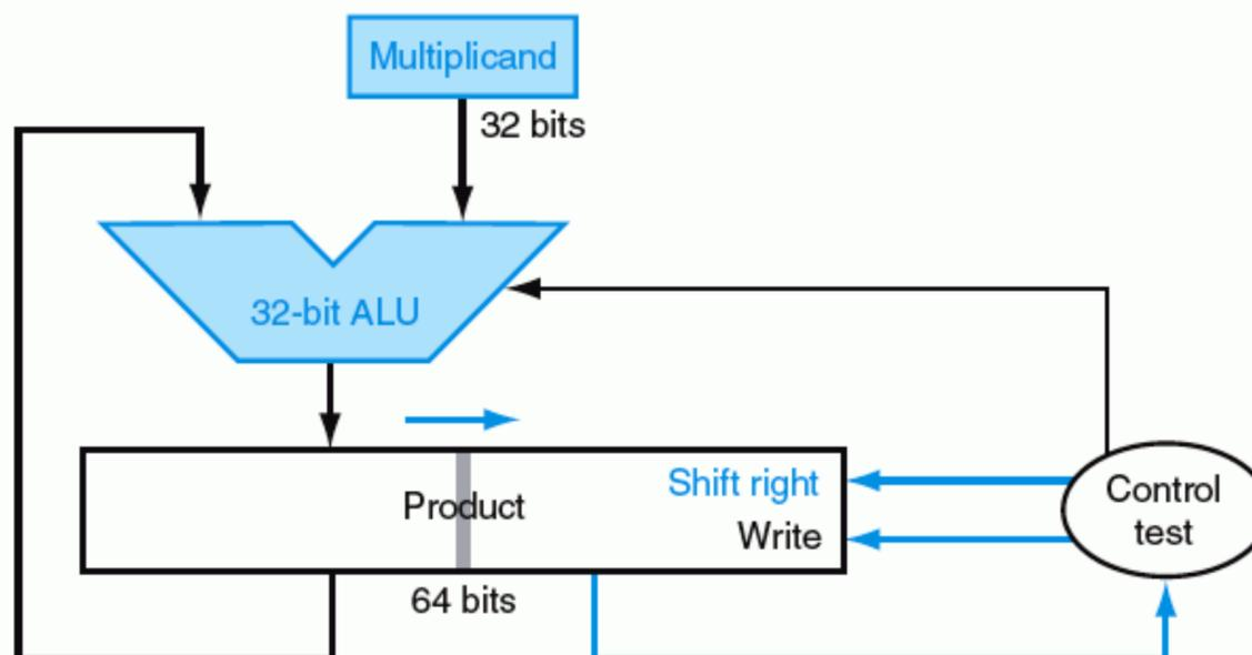
**FIGURE 3.7 Refined version of the multiplication hardware.** Compare with the first version in Figure 3.5. The Multiplicand register, ALU, and Multiplier register are all 32 bits wide, with only the Product register left at 64 bits. Now the product is shifted right. The separate Multiplier register also disappeared. The multiplier is placed instead in the right half of the Product register. These changes are highlighted in color.
