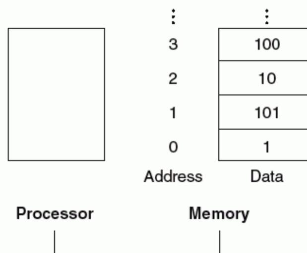
**FIGURE 2.2** Memory addresses and contents of memory at those locations. This is a simplification of the MIPS addressing; Figure 2.3 shows the actual MIPS addressing for sequential word addresses in memory.
