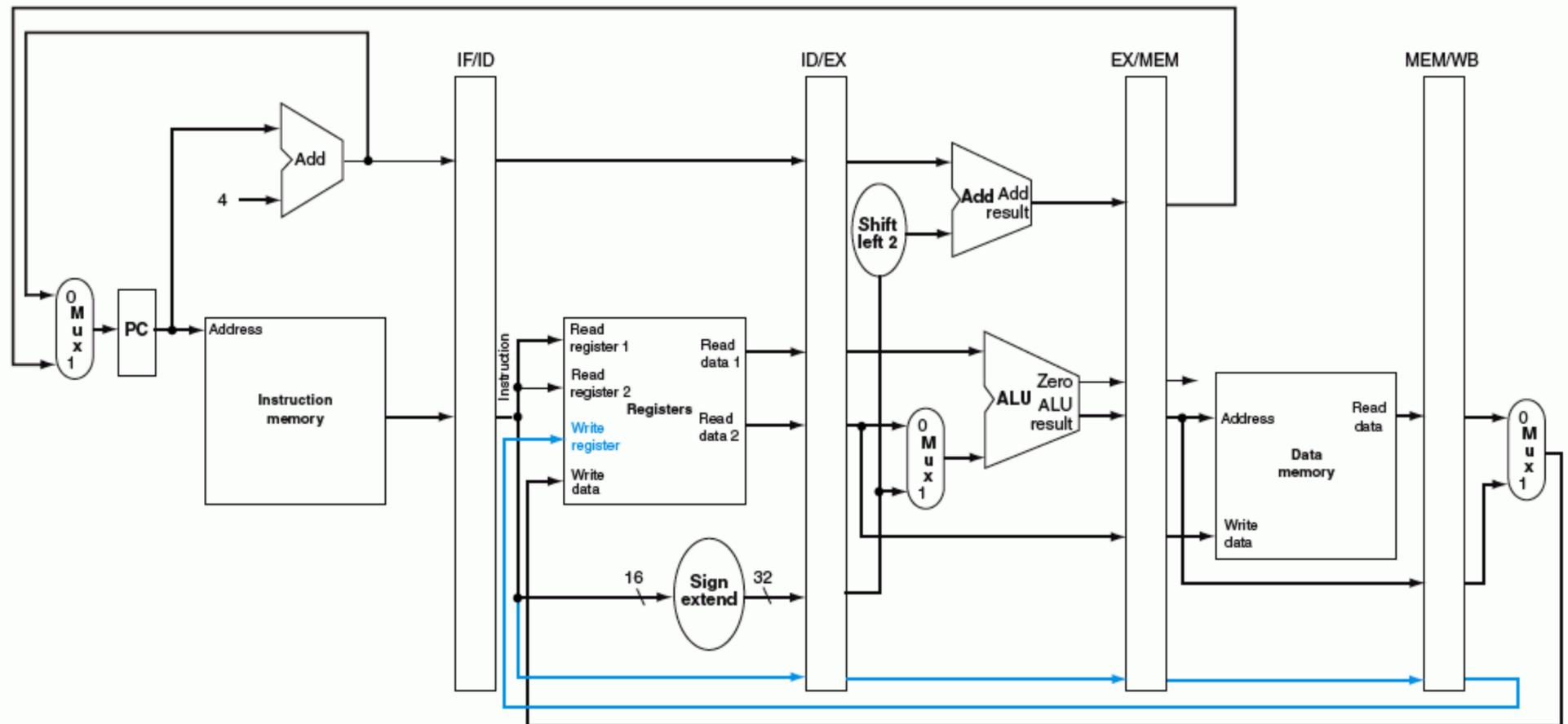
**FIGURE 6.17** The corrected pipelined datapath to properly handle the load instruction. The write register number now comes from the MEM/WB pipeline register along with the data. The register number is passed from the ID pipe stage until it reaches the MEM/WB pipeline register, adding 5 more bits to the last three pipeline registers. This new path is shown in color.
