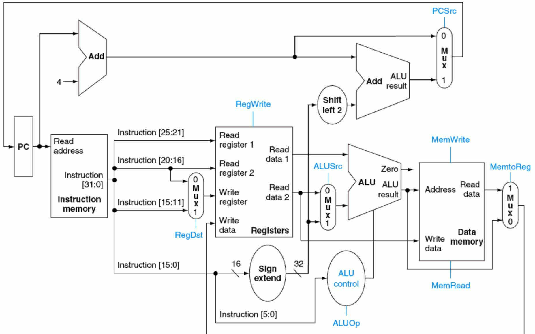
**FIGURE 5.15** The datapath of Figure 5.12 with all necessary multiplexors and all control lines identified. The control lines are shown in color. The ALU control block has also been added. The PC does not require a write control, since it is written once at the end of every clock cycle; the branch control logic determines whether it is written with the incremented PC or the branch target address.
