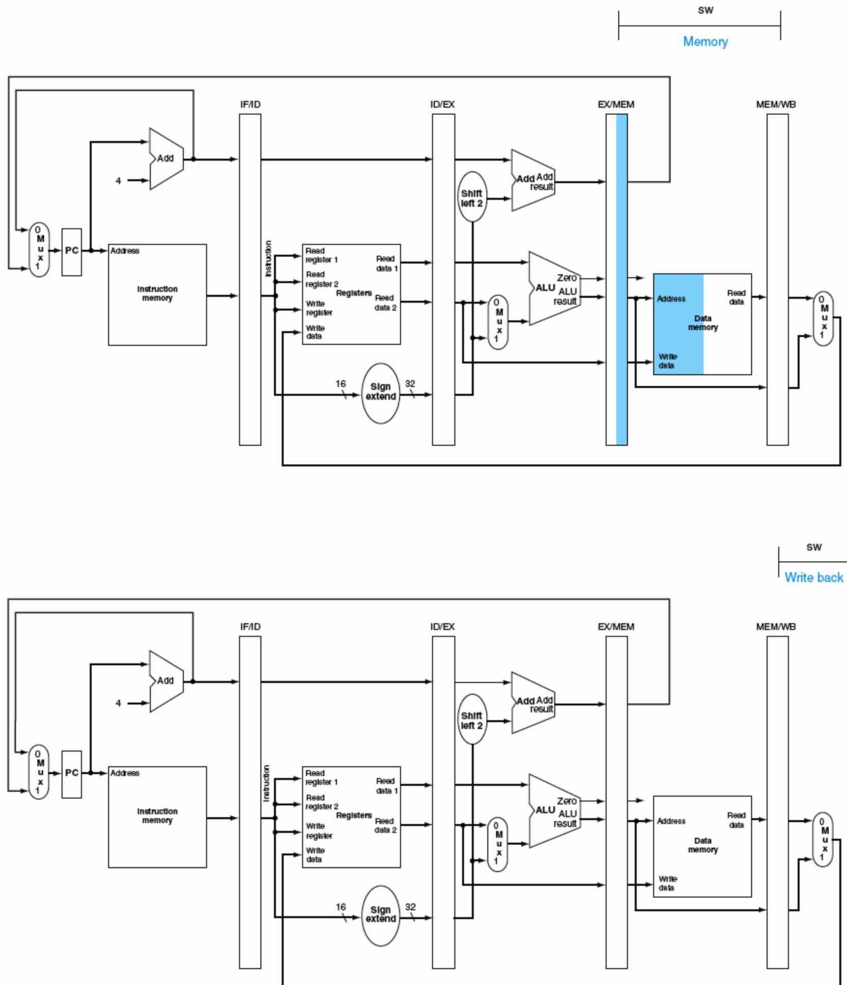
**FIGURE 6.16 MEM and WB: the fourth and fifth pipe stage of a store instruction.** In the fourth stage, the data is written into data memory for the store. Note that the data comes from the EX/MEM pipeline register and that nothing is changed in the MEM/WB pipeline register. Once the data is written in memory, there is nothing left for the store instruction to do, so nothing happens in stage 5.
