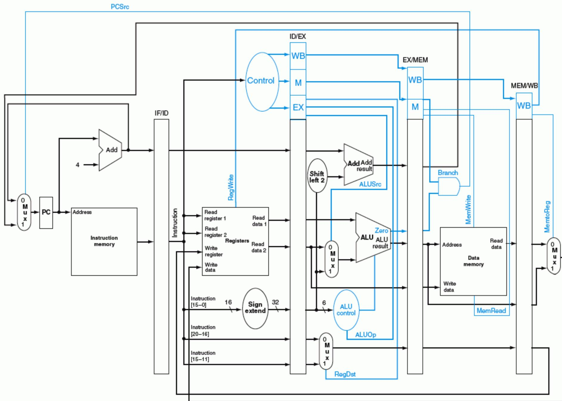
**FIGURE 6.27** The pipelined datapath of Figure 6.22, with the control signals connected to the control portions of the pipeline registers. The control values for the last three stages are created during the instruction decode stage and then placed in the ID/EX pipeline register. The control lines for each pipe stage are used, and remaining control lines are then passed to the next pipeline stage.
