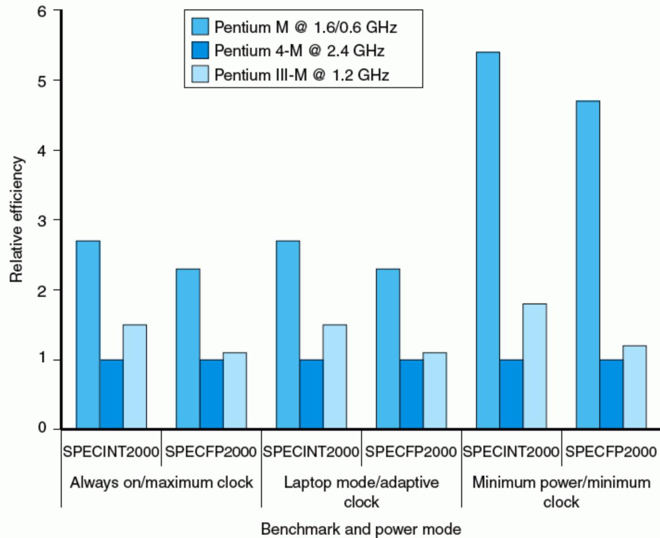
**FIGURE 4.9** The relative energy efficiency of three mobile Pentium processors running SPEC2000 in three modes. Energy efficiency is measured as the inverse of joules consumed per benchmark, which is computed by dividing the inverse of the execution time for a benchmark by the watts dissipated.
