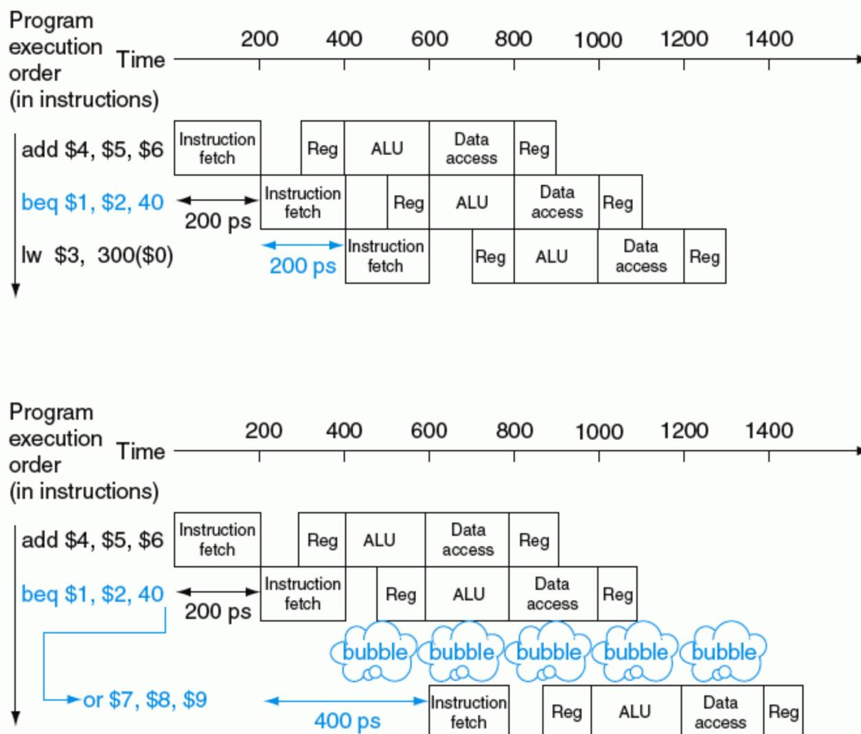
**FIGURE 6.8 Predicting that branches are not taken as a solution to control hazard.** The top drawing shows the pipeline when the branch is not taken. The bottom drawing shows the pipeline when the branch is taken. As we noted in Figure 6.7, the insertion of a bubble in this fashion simplifies what actually happens, at least during the first clock cycle immediately following the branch. Section 6.6 will reveal the details.
