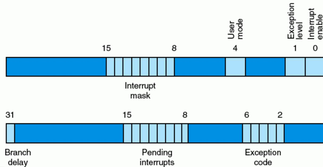
**FIGURE 8.13 The Cause and Status registers.** This version of the Cause register corresponds to the MIPS-32 architecture. The earlier MIPS I architecture had three nested sets of kernel/user and interrupt enable bits to support nested interrupts. Section A.7 in [Appendix A](#) has more details about these registers.
