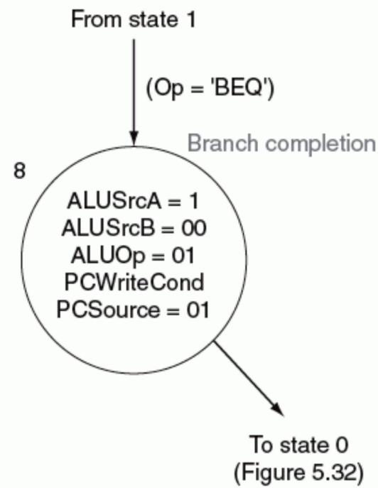
**FIGURE 5.35 The branch instruction requires a single state.** The first three outputs that are asserted cause the ALU to compare the registers (ALUSrcA, ALUSrcB, and ALUOp), while the signals PCSource and PCWriteCond perform the conditional write if the branch condition is true. Notice that we do not use the value written into ALUOut; instead, we use only the Zero output of the ALU. The branch target address is read from ALUOut, where it was saved at the end of state 1.
