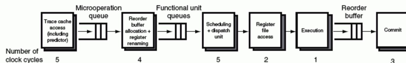
**FIGURE 6.51 The Pentium 4 pipeline showing the pipeline flow for a typical instruction and the number of clock cycles for the major steps in the pipeline.** The major buffers where instructions wait are also shown.
