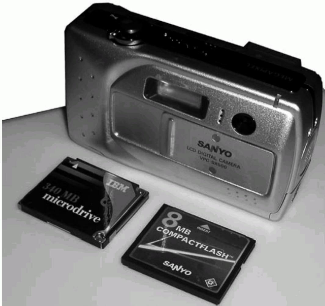
**FIGURE 8.14** The Sanyo VPC-SX500 with Flash memory card and IBM Microdrive.
