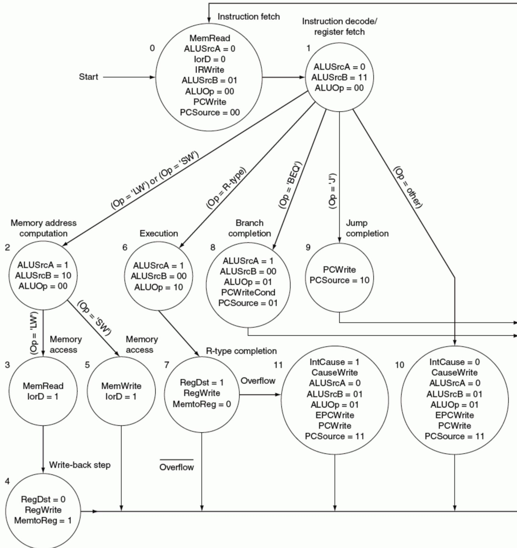
**FIGURE 5.40** This shows the finite state machine with the additions to handle exception detection. States 10 and 11 are the new states that generate the appropriate control for exceptions. The branch out of state 1 labeled (*Op = other*) indicates the next state when the input does not match the opcode of any of *lw*, *sw*, *o* (R-type), *j*, or *beq*. The branch out of state 7 labeled *Overflow* indicates the action to be taken when the ALU signals an overflow.
