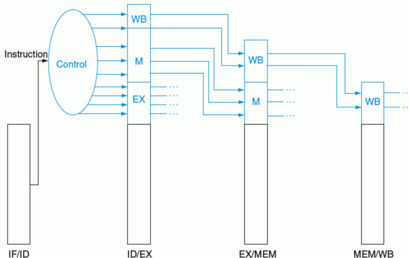
**FIGURE 6.26** The control lines for the final three stages. Note that four of the nine control lines are used in the EX phase, with the remaining five control lines passed on to the EX/MEM pipeline register extended to hold the control lines; three are used during the MEM stage, and the last two are passed to MEM/WB for use in the WB stage.
