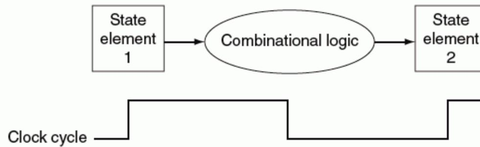
**FIGURE 5.3 Combinational logic, state elements, and the clock are closely related.** In a synchronous digital system, the clock determines when elements with state will write values into internal storage. Any inputs to a state element must reach a stable value (that is, have reached a value from which they will not change until after the clock edge) before the active clock edge causes the state to be updated. All state elements, including memory, are assumed to be edge-triggered.
