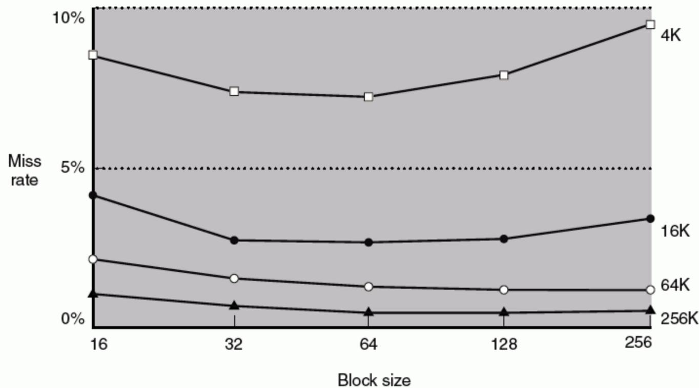
**FIGURE 7.8 Miss rate versus block size.** Note that miss rate actually goes up if the block size is too large relative to the cache size. Each line represents a cache of different size. (This figure is independent of associativity, discussed soon.) Unfortunately, SPEC2000 traces would take too long if block size were included, so these data are based on SPEC92.
