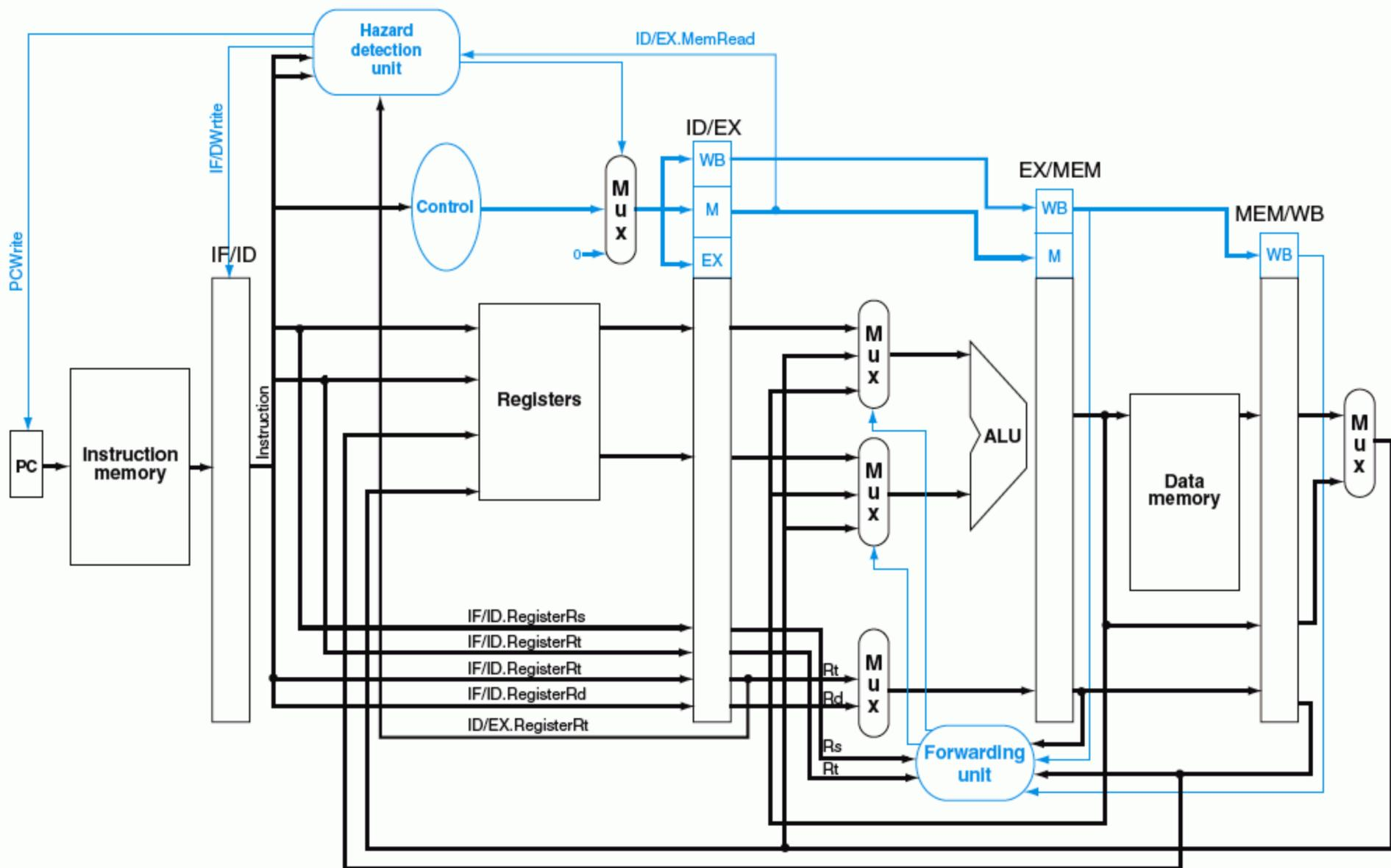
**FIGURE 6.36** Pipelined control overview, showing the two multiplexers for forwarding, the hazard detection unit, and the forwarding unit. Although the ID and EX stages have been simplified—the sign-extended immediate and branch logic are missing—this drawing gives the essence of the forwarding hardware requirements.
