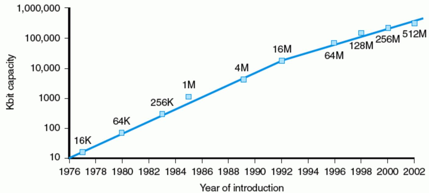
**FIGURE 1.13 Growth of capacity per DRAM chip over time.** The  $y$ -axis is measured in Kbits, where  $K = 1024$  ( $2^{10}$ ). The DRAM industry quadrupled capacity almost every 3 years, a 60% increase per year, for 20 years. This “four times every three years” estimate was called the *DRAM growth rule*. In recent years, the rate has slowed down somewhat and is somewhat closer to doubling every two years or four times every four years.
