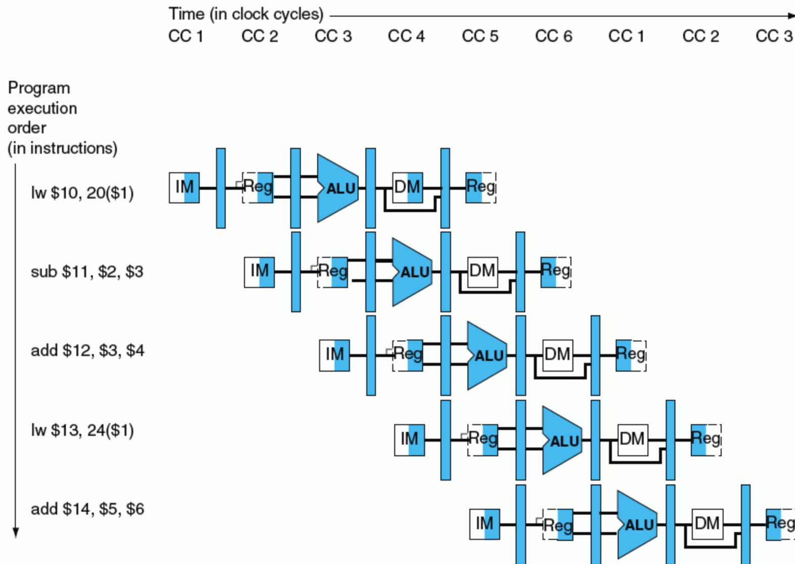
**FIGURE 6.19 Multiple-clock-cycle pipeline diagram of five instructions.** This style of pipeline representation shows the complete execution of instructions in a single figure. Instructions are listed in instruction execution order from top to bottom, and clock cycles move from left to right. Unlike Figure 6.4, here we show the pipeline registers between each stage. Figure 6.20 shows the traditional way to draw this diagram.
